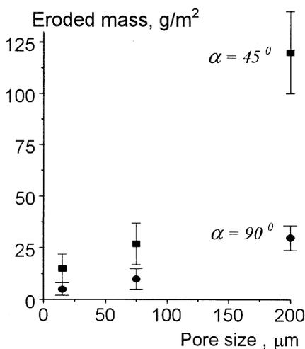
Fig. 1. Lithium mass loss vs CPS effective pore size (disruption simulation experiment at 5 MJ/m<sup>2</sup>, pulse duration 200–500  $\mu\text{s}$ , hydrogen plasma),  $\alpha$ -plasma flow incidence angle.
