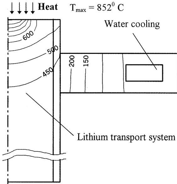
Fig. 8. Temperature field in the lithium target in steady state at  $10 \text{ MW/m}^2$ . Target diameter is 40 mm, heat loaded area diameter is 18 mm, heat sink is provided by water cooling through the cavity in flange.
