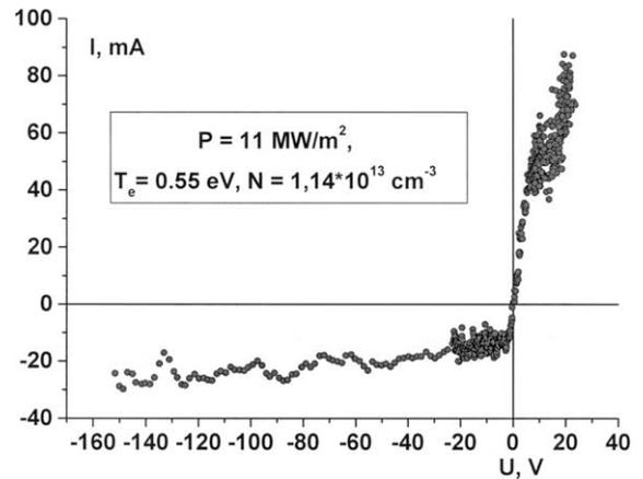
Fig. 7. Voltage–current characteristics of a single Langmuir probe taken in steady-state lithium plasma (heat flux and corresponding plasma parameters are shown).
