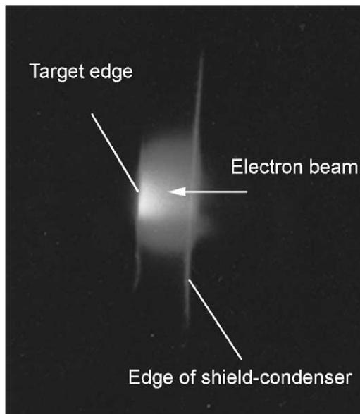
Fig. 6. Photo of lithium plasma near lithium CPS target at 4 MW/m<sup>2</sup> of incident power flux.
