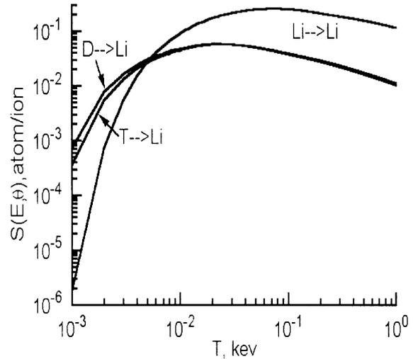
Fig. 9. Physical sputtering of lithium surface by hydrogen, deuterium and lithium ions (calculated values average over ion energy and incident angle,  $\delta = Z_1 e \phi / T_i = 3$ , Mach number = 1).
