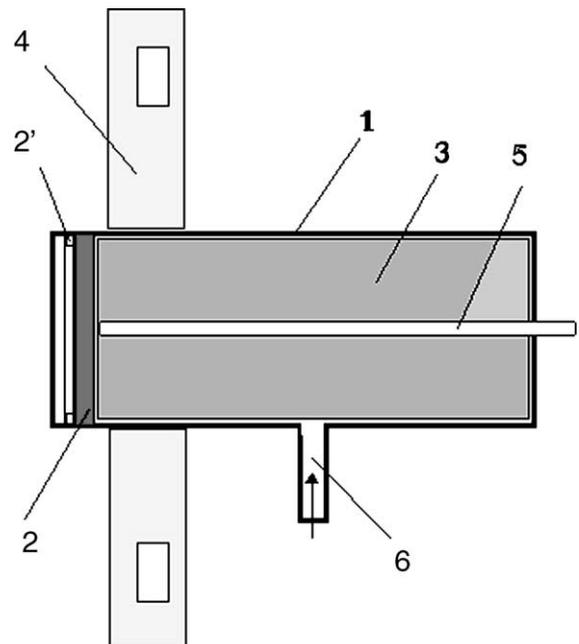
Fig. 2. Lithium target with CPS: 1 – casing; 2 – CPS ( $d = 40$  mm); 2' – clamp; 3 – transport structure; 4 – water cooled flange; 5 – thermocouple; 6 – lithium supply.
