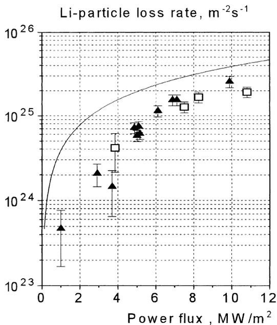
Fig. 3. Measured lithium loss rate versus incident power flux for two capillary structures: solid symbols – mesh  $h = 0.15$  mm, open symbols – perforated plate  $r = 0.3$  mm. The curve shows calculation of maximum lithium mass loss when the incident power is totally going to evaporation.
