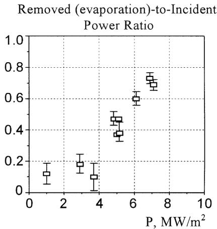
Fig. 5. Efficiency of heat removal from CPS target via evaporation vs incident power flux.
