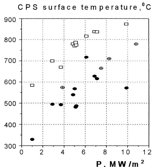
Fig. 4. Temperature at the CPS target surface as measured by thermocouple (closed circles – mesh, open circles – perforated plate) and deduced from lithium mass balance (squares).
