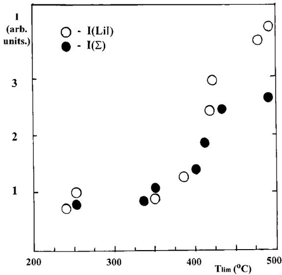
Fig. 6. Total light and LiI intensity as function of current CPS temperature  $T_{lim}$ .
