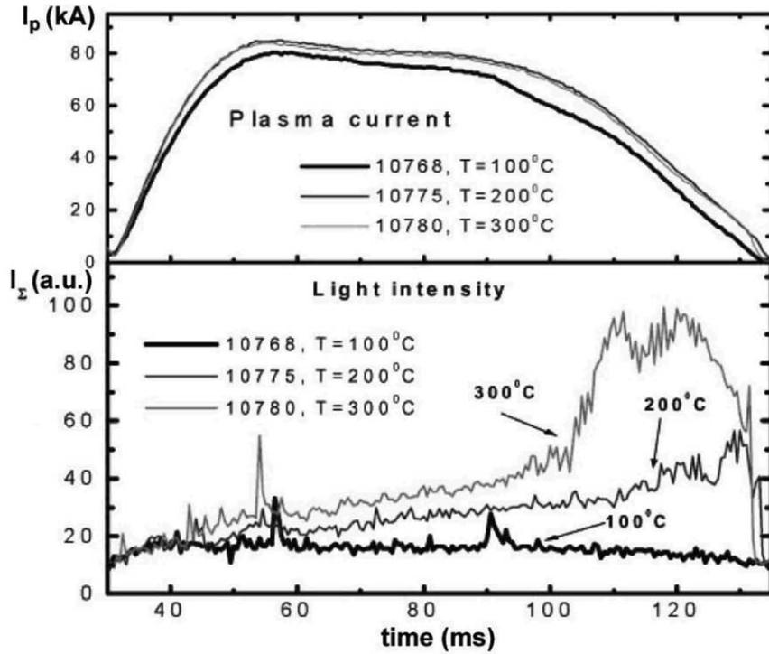
Fig. 5. Temporal behavior of integral light emission from the lithium limiter for different initial temperatures (100–300 °C).
