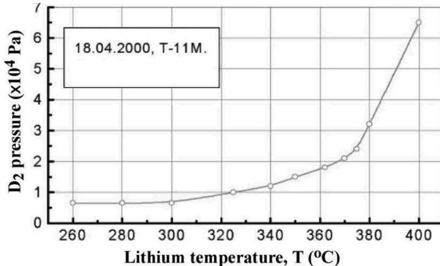
Fig. 9. Evaluation of D<sub>2</sub> pressure in the tokamak chamber during lithium limiter heating after D<sub>2</sub>-discharge operations.
