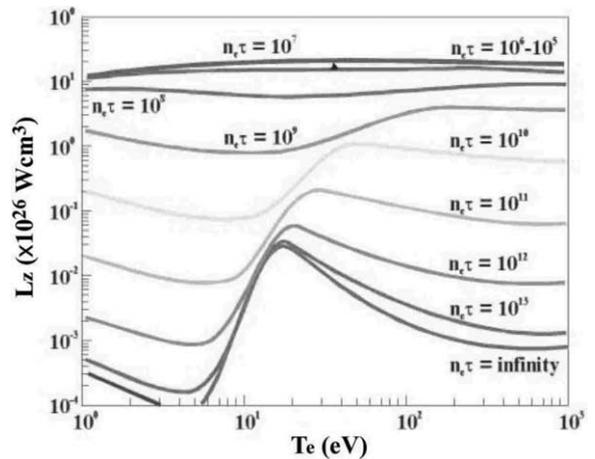
Fig. 7. Lithium radiation rate as function of  $n_e \tau$  and  $T_e$ .
