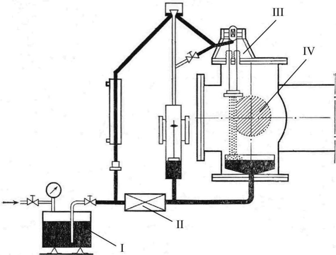
Fig. 1. Scheme of T-3M liquid gallium jet-drop limiter. I: gallium reservoir; II: MHD-pump; III: MHD shaper; IV: plasma column.
