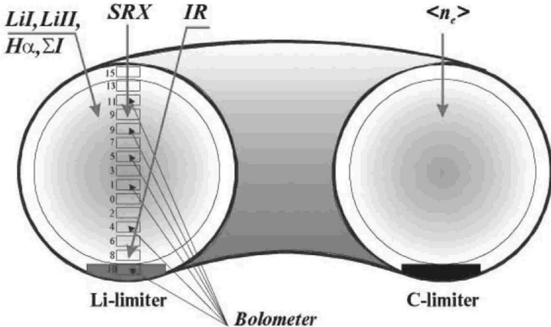
Fig. 3. Scheme of the T-11M experiment with lithium CPS-limiter. 1–15, fast bolometer measurement channels; IR, channel of infrared measurements; SXR, soft X-ray measurements channels; LiI, LiII,  $H\alpha$ ,  $\Sigma I$ , spectral line and total light measurements channels;  $n_e$ , electron density micro-wave measurements.
