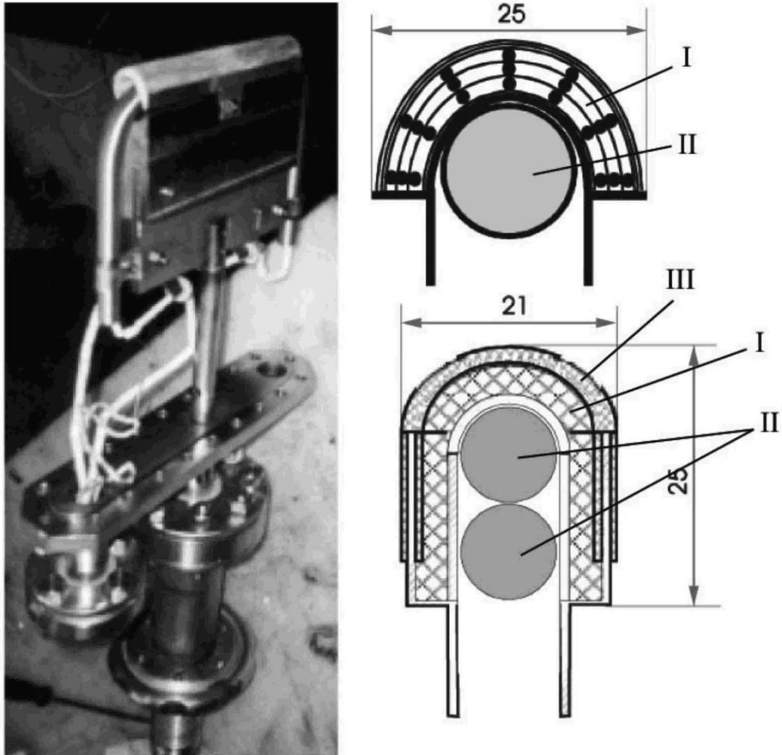
Fig. 4. Lithium rail limiter: (a) general view; (b) CPS lithium limiter (cross-section); I: CPS layer with pore radius 100  $\mu\text{m}$ ; II: limiter pre-heaters; III: CPS layer with pore radius 30  $\mu\text{m}$ . All dimensions are in mm.
