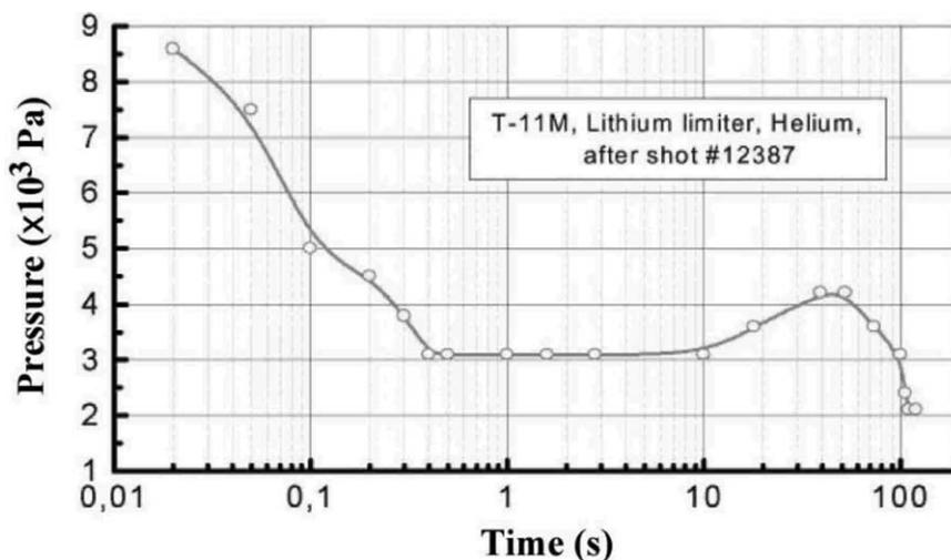
Fig. 8. Temporal behavior of He pressure in the tokamak chamber after helium discharge (pump speed is decreased).
