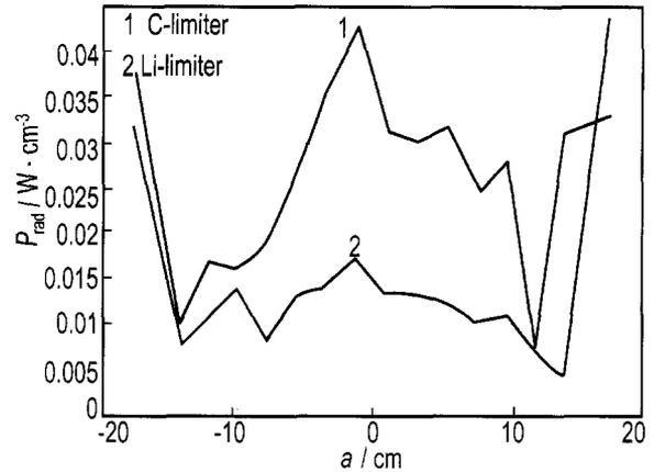
Fig.5 Radiation losses profile for shots with lithium and graphite limiters
