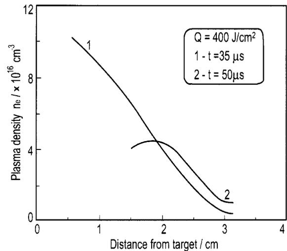
**Fig.1** Plasma density distribution near the target
