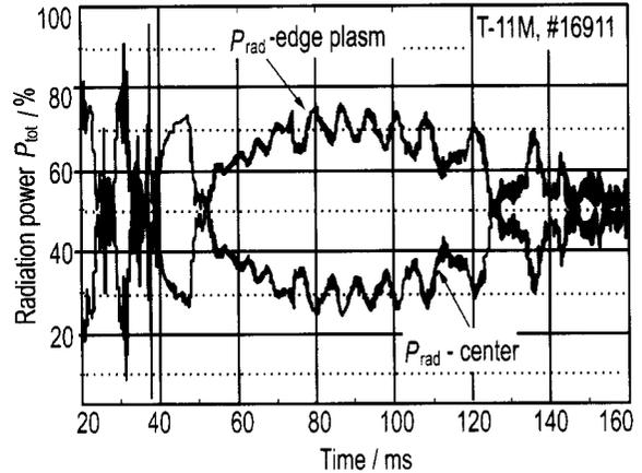
**Fig.3** Behavior of relative radiation losses in discharge with “hot” lithium by limiter( $400^\circ\text{C}$ ) from central ( $r < 15.2$  cm) and peripheral plasma ( $r > 15.2$  cm)
