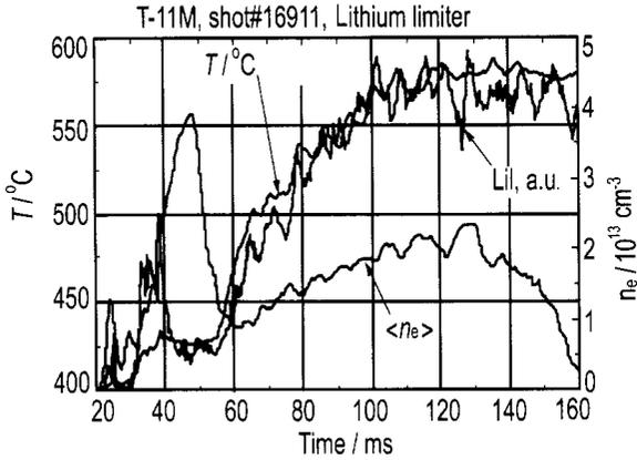
**Fig.2** The temporal behavior of limiter surface temperature LiI line and electron density
