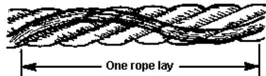
Figure 1-2. Rope Lay
