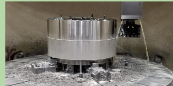
At GJ Oliver: Mandrel Fabrication
