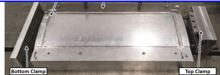
Distortion Control Weld Fixture for Slings
