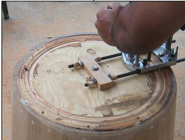
Axis-centered router cutting guide.
