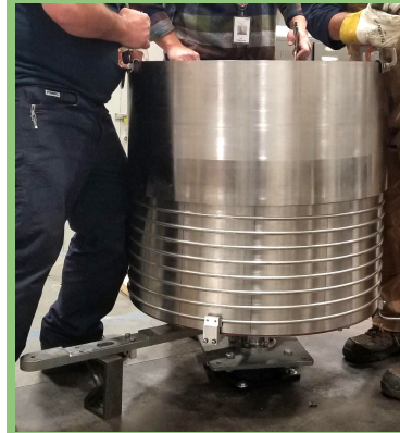
At PPPL C-MG: Preparing HTT for Heat Treatment
