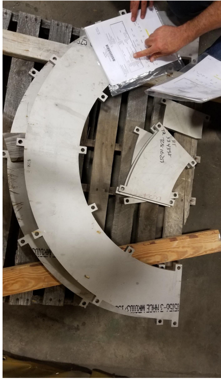
HTP Inconel 625 Plates after Water-Jetting
