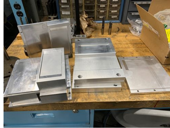
Machined epoxy pad casting molds
