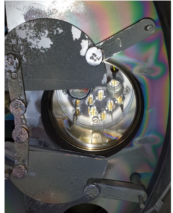
Aerodag sprayed on Synthetic Aperture Microwave Imaging (SAMI) shutter
