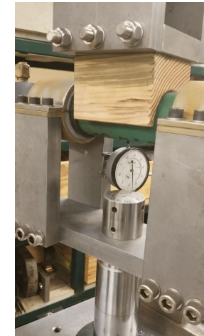
Fixture on the 10kip MTS Machine with 4.25in Wood Saddle applying distributed load.
