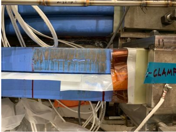
Preparation of the PF-4/5 coils surfaces to accept the epoxy pads
