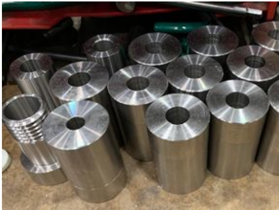
In-process fabrication of the Belleville washer housing assemblies
