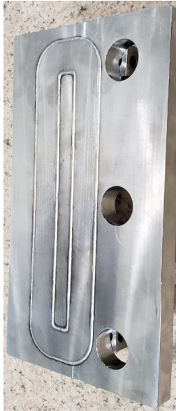
First Machining and EB Welded
