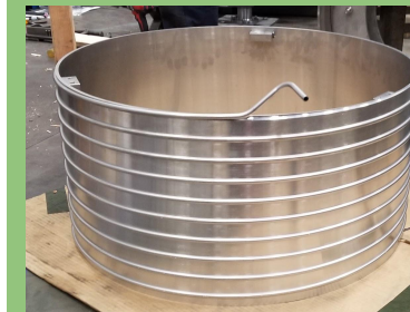
At PPPL C-MG: HTT after Bending Procedure
