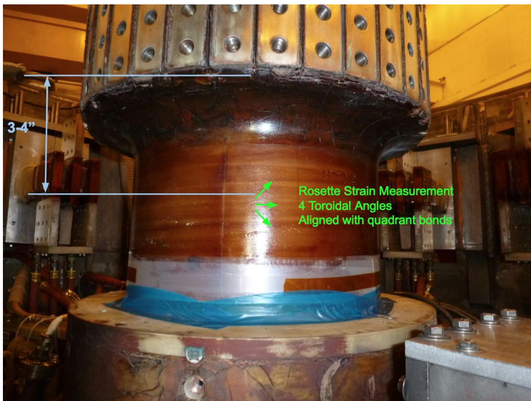
Fig. 4.6-1: Locations of the TF twist measurements on the upper part of the bundle.
