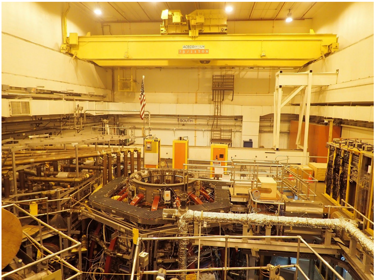
Figure 2-6: View to the south from NB #2, viewing the NSTX-U device and into the south high bay over the south shield wall. The large mobile door on the right in the south high bay provides access to the TFTR test cell.
