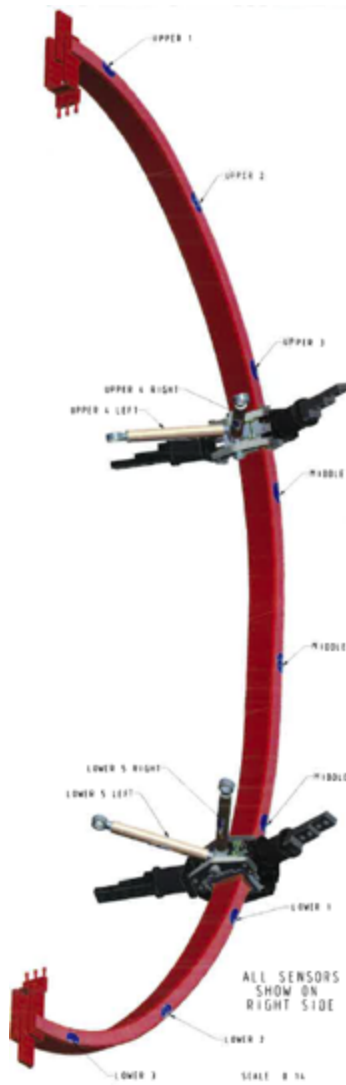
Figure 4. TF Outer Leg with attached strain gauges
