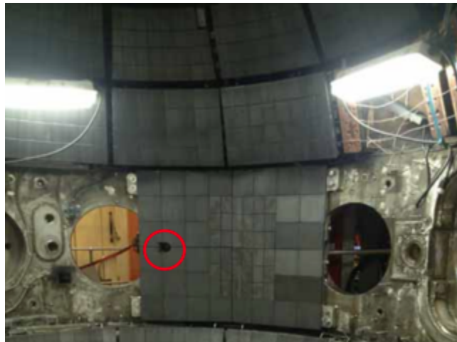
Figure 10. MSE-LIF Gap in Neutral Beam Armor
