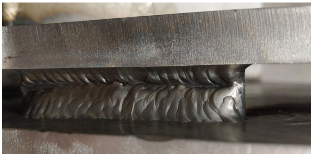
Figure 3: Spacer block weld on test stand (final). Upper weld changed to 3/16"
