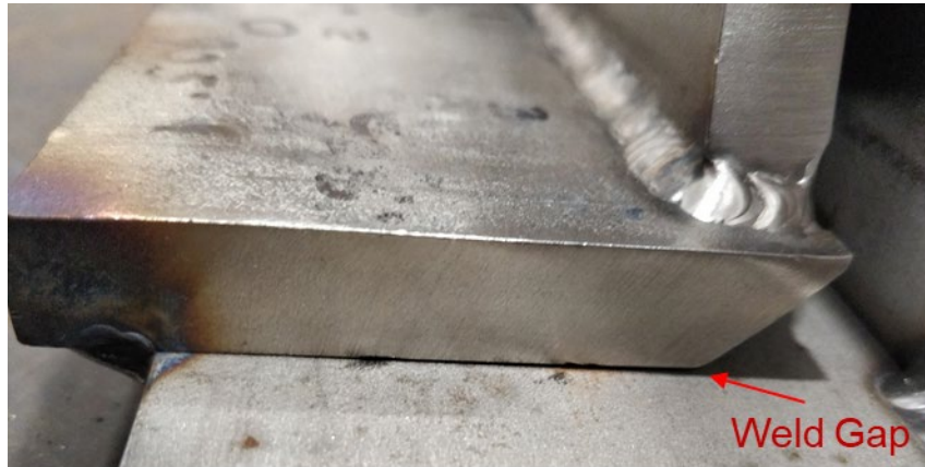
Figure 4: Second trial of weld to test stand
