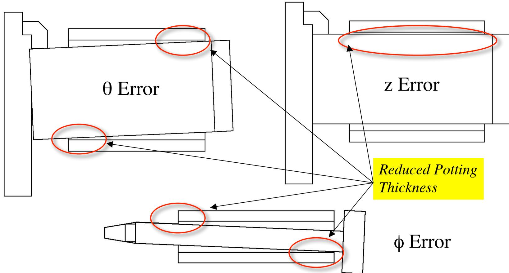
Potting must accommodate dimensional tolerances of flags and conductors while maintaining structural and electrical functions
