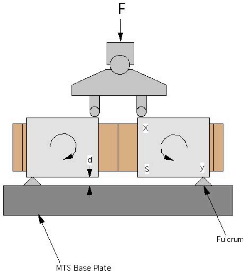
X,Y= sides of box which provide moment reaction in service
