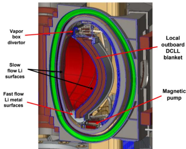
Figure 5 – Cross-sectional image of R=1m, A=2.4 SHPD concept capable of testing vapor box divertors, slow-flow LM first-walls, and fast-flow LM divertors – potentially simultaneously.
