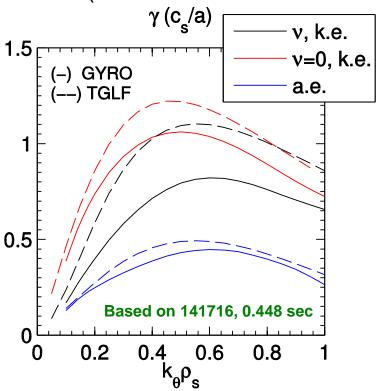
TGLF stabilization with increasing collisionality not as strong as GYRO/GS2 → need to improve trapped electron response
