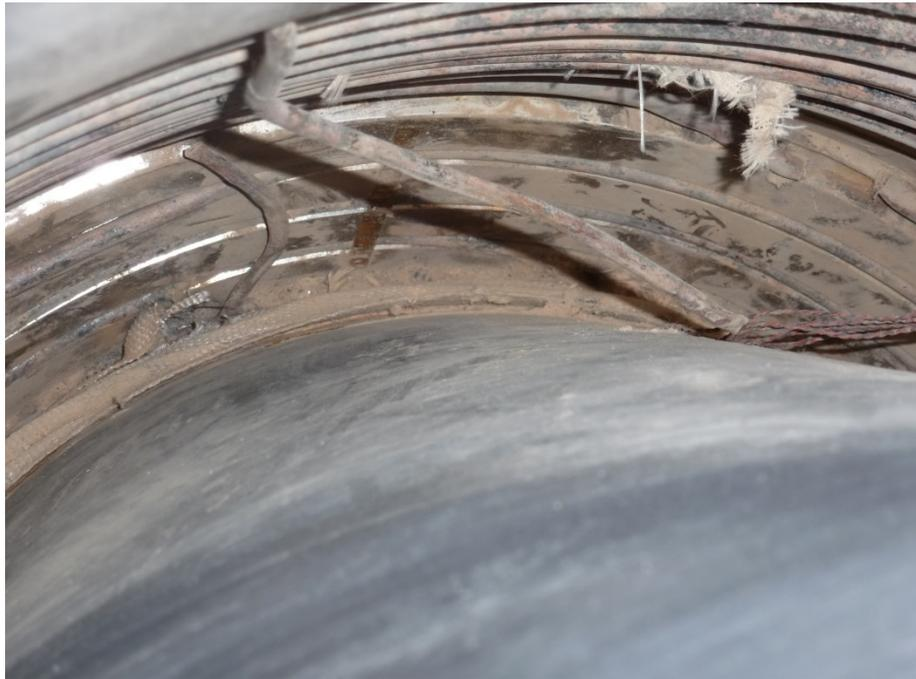
Discovered a Failed Lower Cooling Tube
