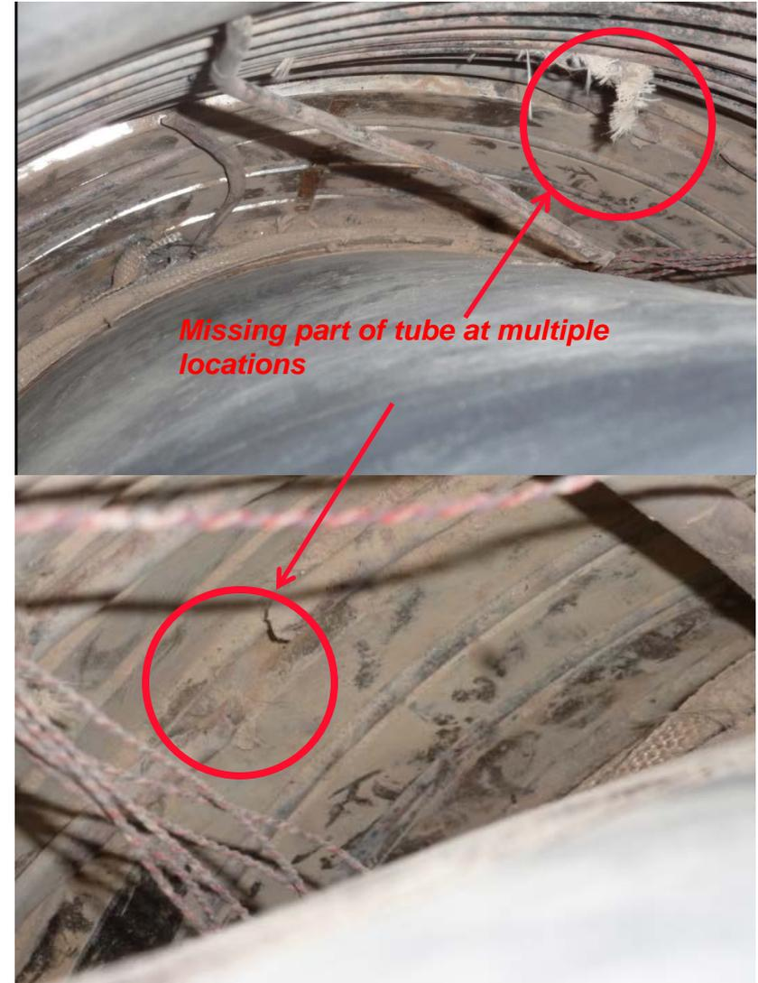
Lower cooling tube also breached → damaged → need to remove both CS and casing to access tube, PF1AL
