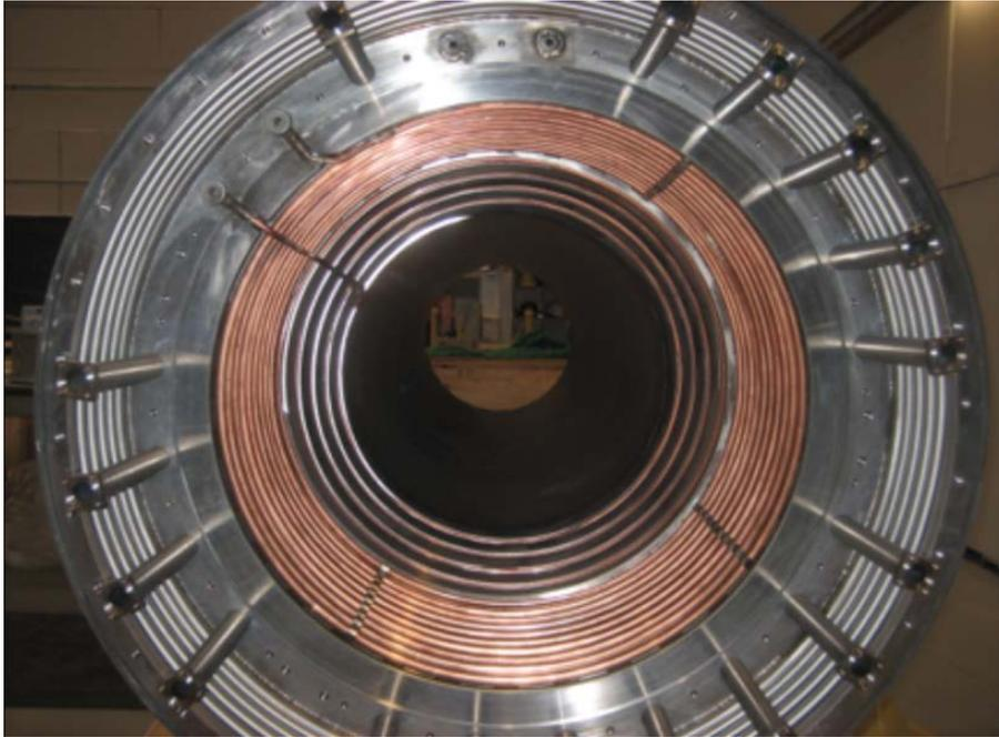
Severe damage in divertor CS cooling tubes
