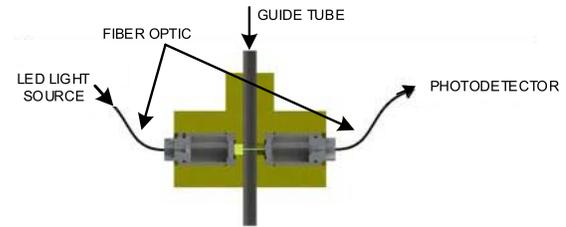
Fig. 3. Granule counter uses light attenuation to photodetector to indicate granule passage, with amplitude related to granule size.
