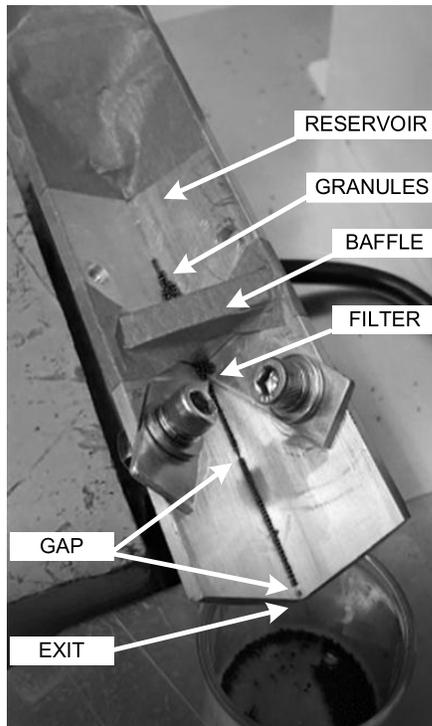
Fig. 2. Large V-groove in-line feeder bench tested successfully at low injection rates 0–60 per second using 0.7-mm carbon granules.
