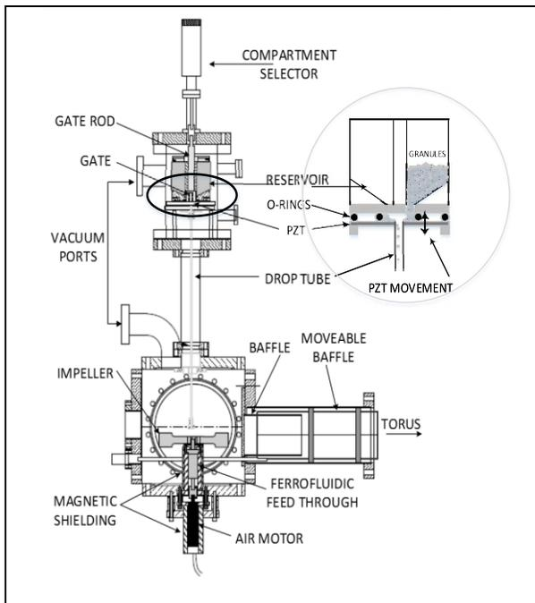
Fig. 1. Original impurity injector created by Mansfield and Roquemore at PPPL used a PZT disk to move granules to the entrance of the drop tube.
