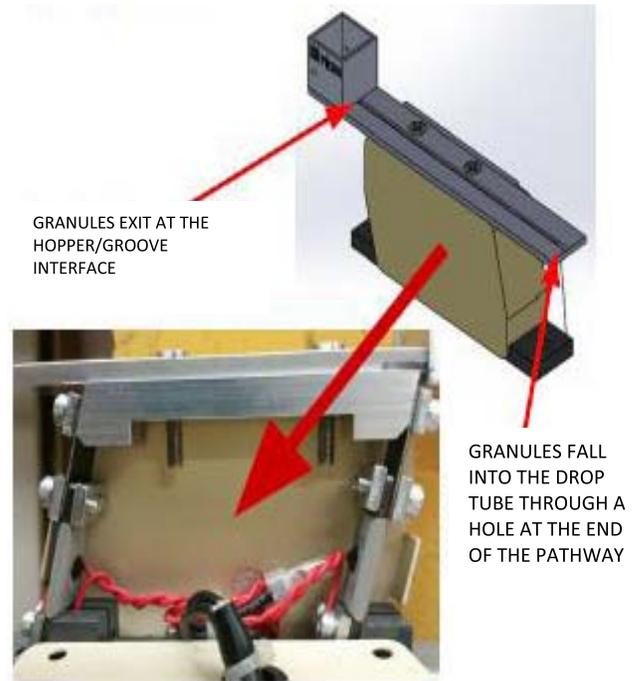
Fig. 4. Second design used the Mirai-Sanki piezoelectric in-line feeder, internal parts shown above, with a storage hopper and small V-groove.
