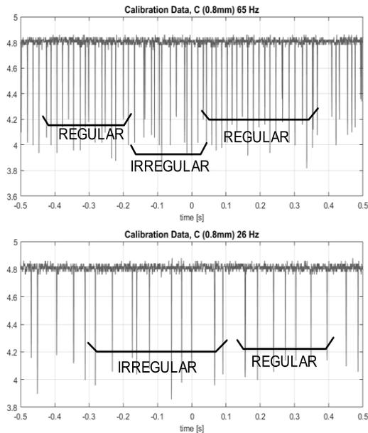
Fig. 7. Granule counter scope traces show zones of regular and irregular periodicity at both low and mid-frequencies.
