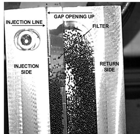
Fig. 9. When feed rates are  $>60$  Hz, gaps form in the feed line causing regular periodicity drift in a cyclic basis, while granule lines without gaps produce a more regular periodicity.
