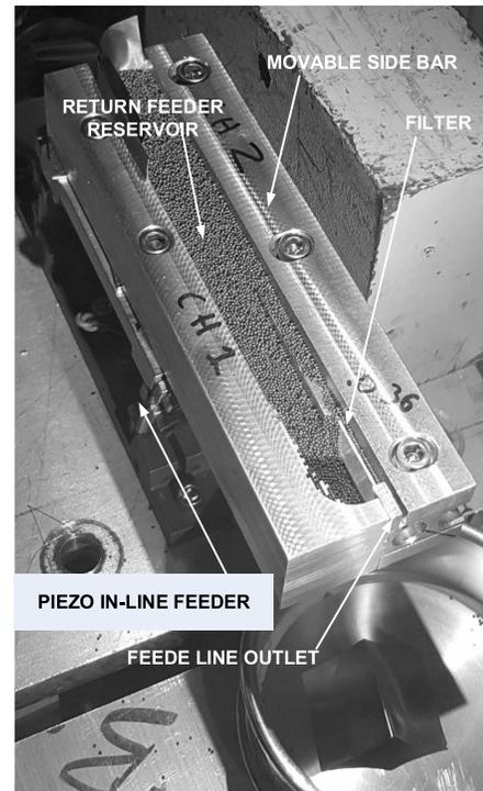
Fig. 6. Final version shown successfully bench testing using 0.7-mm lithium granules in an Argon-filled glove box.
