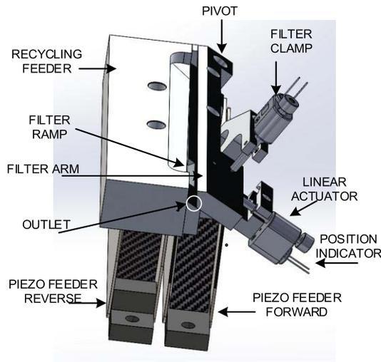
Fig. 10. Final in-line feeder designed for vacuum using piezovacuum compatible actuators and position indicators.
