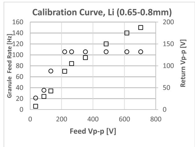
Fig. 8. Calibration curve for lithium injection and the return feeder drive voltage. The return side voltage ramps up faster to keep the feed side full, saturating at  $\sim 200$  Hz.
