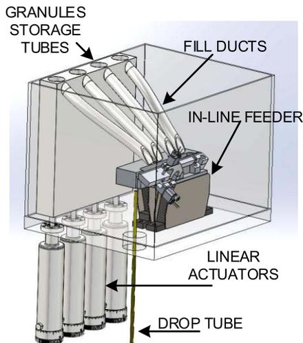
Fig. 11. In-line feeder vacuum assembly design with four material reloading capabilities without a vacuum cycle.
