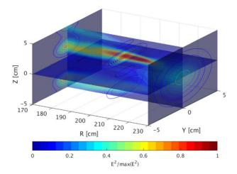
**Figure 13.** 3D EC beam propagation evaluated by the FWR3D with the paraxial approximation with edge density fluctuations  $(\max(\delta n/n) = 20\%)$ . Same beam parameter used in the 2D calculation.
