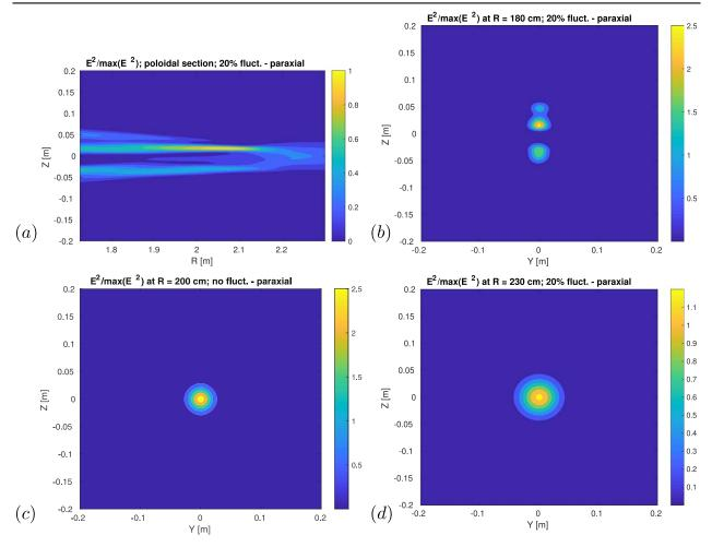
Figure 14. (a) Poloidal section of the 3D EC beam shown in figure 13; cross-sections of the EC beam at three different locations: R = 180 cm (b), R = 200 cm (c), R = 230 cm (d).
