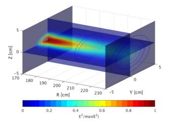
**Figure 11.** 3D EC beam propagation evaluated by the FWR3D with the paraxial approximation without edge density fluctuations. Same beam parameter used in the 2D calculation.
