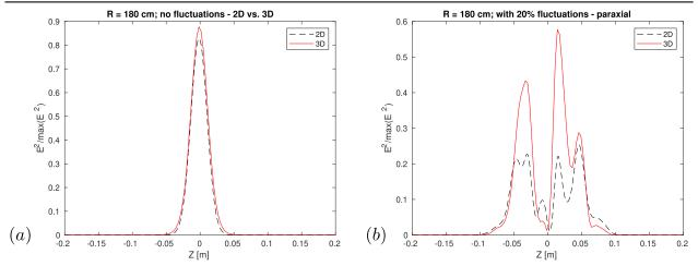
**Figure 15.** (a) Comparison between the beam cross-section evaluated by the 2D (dashed black curve) and the 3D (red curve) codes at R = 180 cm and Y = 0 cm for the case without fluctuations (20%); (b) comparison between the beam cross-section evaluated by the 2D (dashed black curve) and the 3D (red curve) codes at R = 180 cm for the case with fluctuations (20%).
