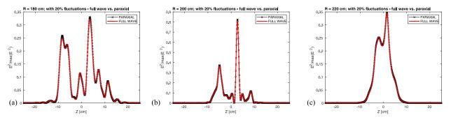
**Figure 6.** Comparison between paraxial (black curves) and full-wave (red curves) methods of the beam cross-sections with the presence of the density fluctuations at three different radial locations, i.e. R = 180 cm (figure (a)), R = 200 cm (figure (b)), and R = 220 cm (figure (c)).
