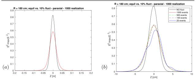
**Figure 10.** (a) Comparison of the beam cross-section at R = 180 cm between the case without fluctuations (black curve) with the averaged solution when 1000 different realization of the density fluctuations are adopted. (b) Convergence test of the average solutions with different number of realizations of density fluctuations (20, 50, 100, 500, and 1000 realizations).
