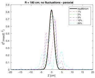
**Figure 8.** Beam cross-section for the cases shown in figure 7 at R = 180 cm. The bold black curve represents the equilibrium case.
