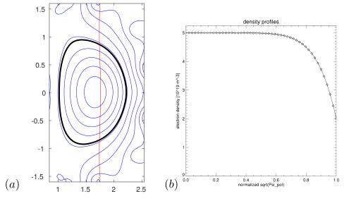
Figure 1. (a) Magnetic flux surfaces equilibrium used in the simulations. The bold black curve represents the last closed flux surface and the red line is the 2nd electron cyclotron harmonic. (b) The electron density as a function of the square root of the normalized poloidal flux.
