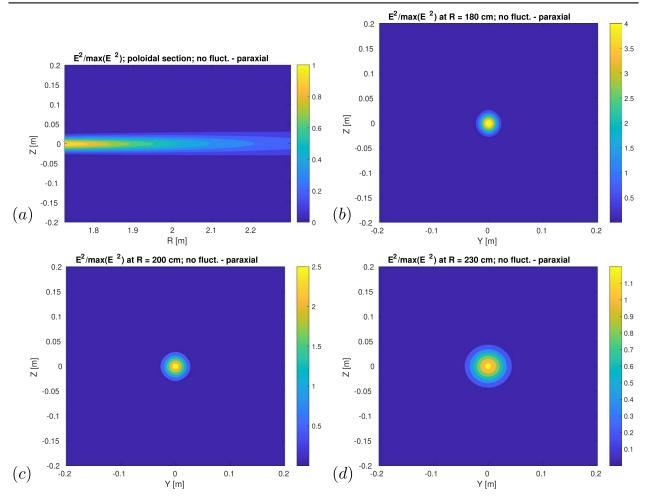
Figure 12. (a) Poloidal section of the 3D EC beam shown in figure 11; cross-sections of the EC beam at three different loations: R = 180 cm (b), R = 200 cm (c), R = 230 cm (d).
