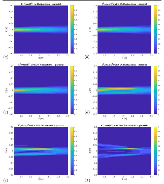
Figure 7. 2D EC beam propagation with no density fluctuations in figure (a) and different density fluctuations with maximum values of 1% (figure (b)), 2% (figure (c)), 5% (figure (d)), 10% (figure (e)), and 20% (figure (f)).
