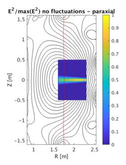
Figure 3. The EC divergent beam propagation with the magnetic flux surfaces in black and the 2nd EC harmonic in red.
