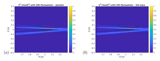
**Figure 5.** 2D EC beam propagation evaluated by the paraxial (figure (a)) and the full-wave (figure (b)) methods in the presence of the density fluctuations shown in figure 2 with  $\max(\delta n/n) = 20\%$ .
