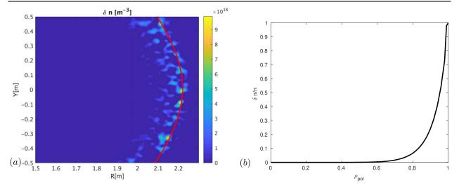
Figure 2. (a) 2D density fluctuations used in the simulations where the red curve represents the last closed flux surface. (b) The normalized density fluctuations as a function of the square root of the normalized poloidal flux.
