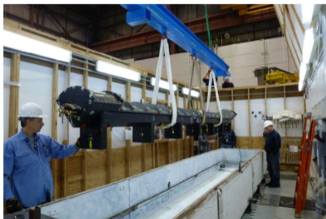
TF Quadrant VPI mold lowered into the oven.
