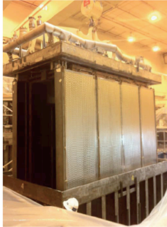
2 nd NBI lid with the cryo-panel being lowered into the beam box in the NSTX-U Test Cell.
