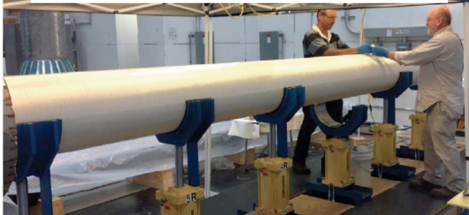
Inner TF bundle with ground wrapping before VPI
