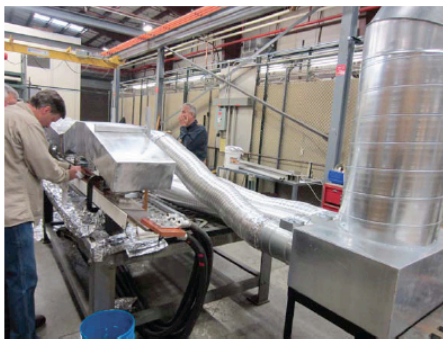
TF conductor soldering station
