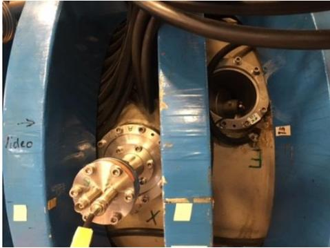
**Above:** Installed edge Langmuir probe and camera 2.
