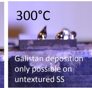
For both experiments, all surface texturing tested were totally liquid metal phobic and no contact angles have been measured.
