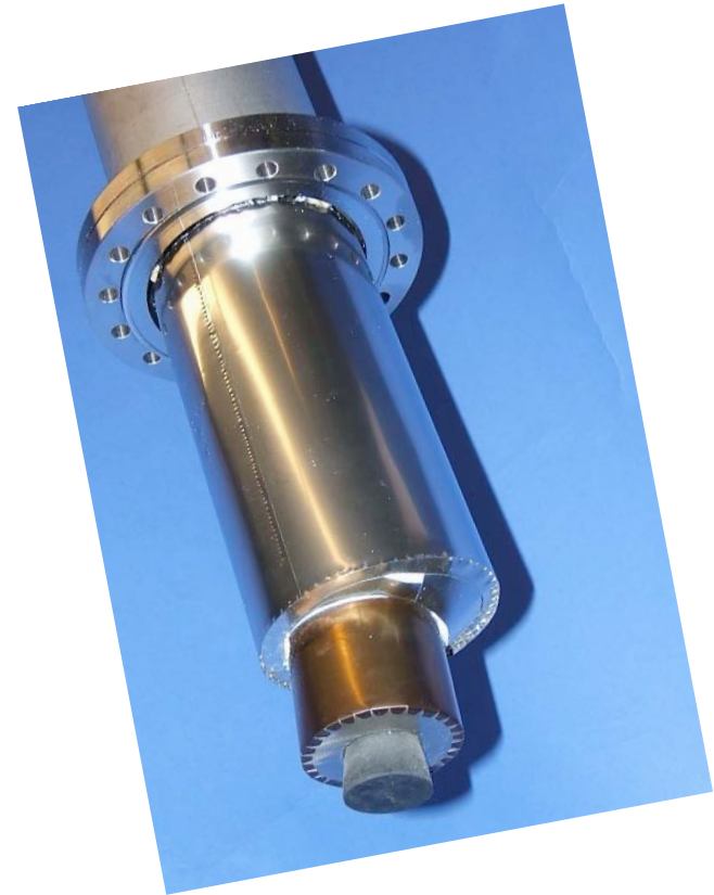
LITER on movable probe, loaded with Li under argon
