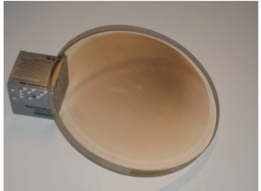
Photograph of the MPTS viewing window after the end of the 2007 run campaign
