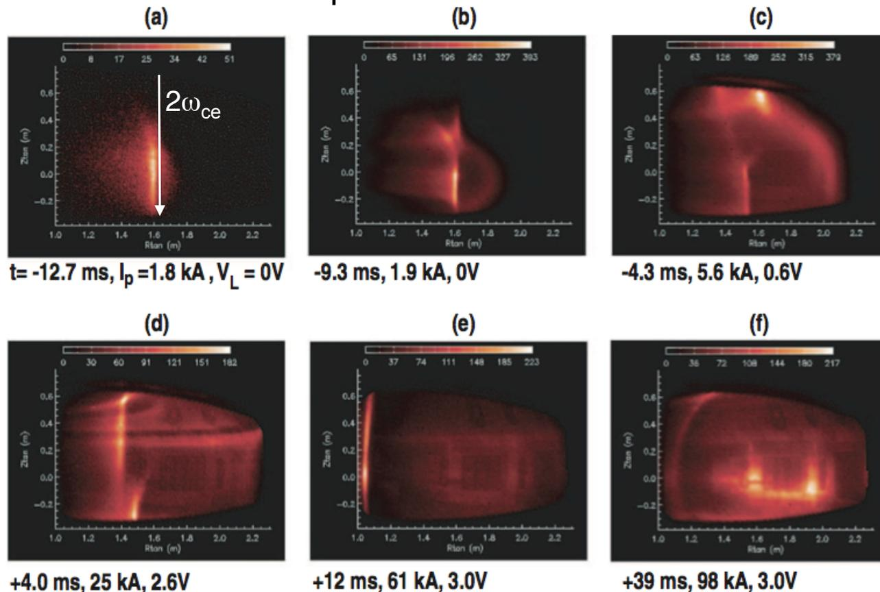
Fast-framing camera of  $\text{C}^{\text{III}}$  emission during 2<sup>nd</sup> harmonic ECH in DIII-D
