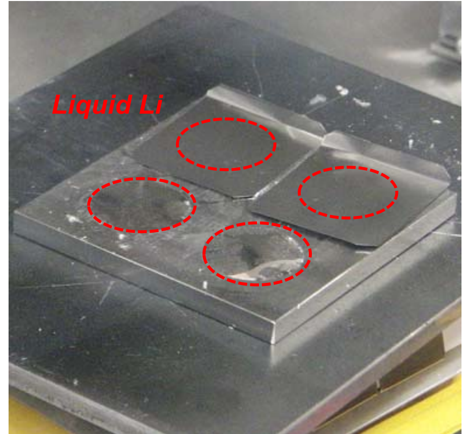
Four Li samples melted into wells on a SS prototype plate (two with shim stock covers)
