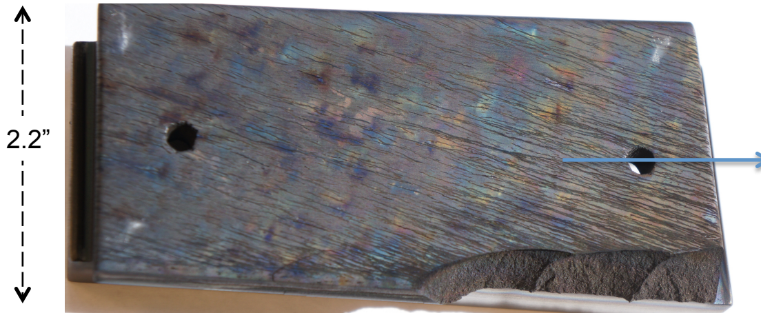
NSTX-U upper divertor graphite tile with arc tracks
