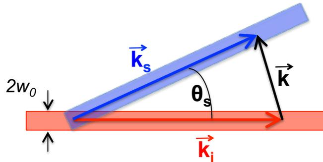
$k$  of the turbulence is selected by geometry.
