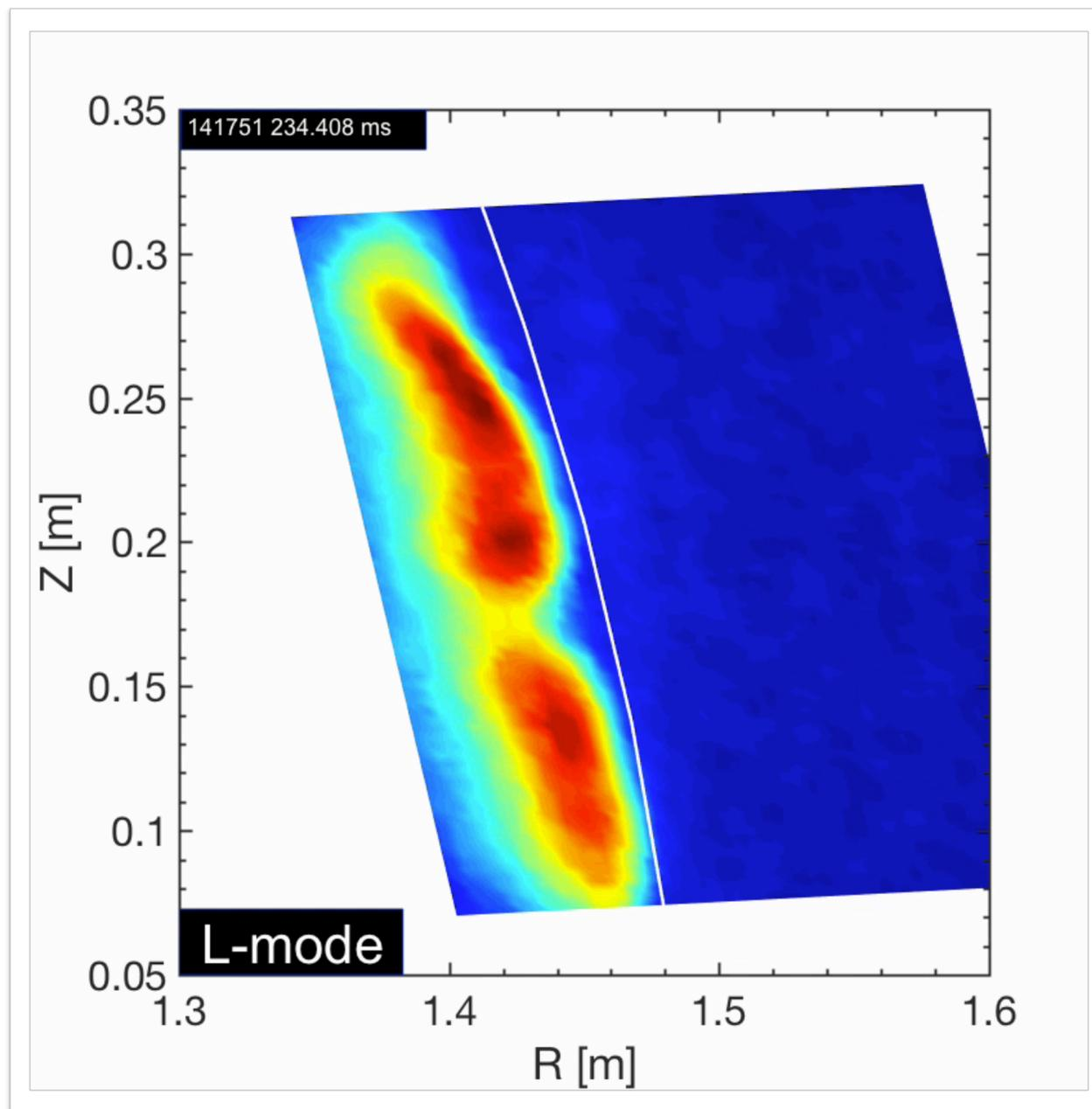
**GPI provides edge turbulence images**
