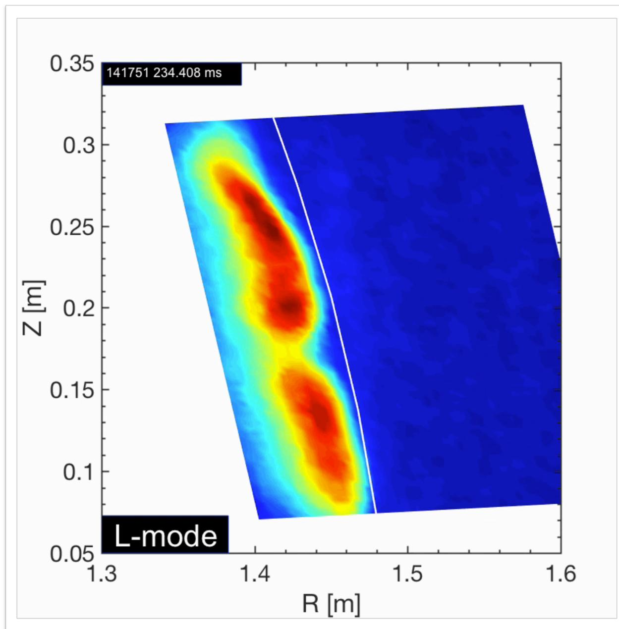
**GPI provides edge turbulence images**
