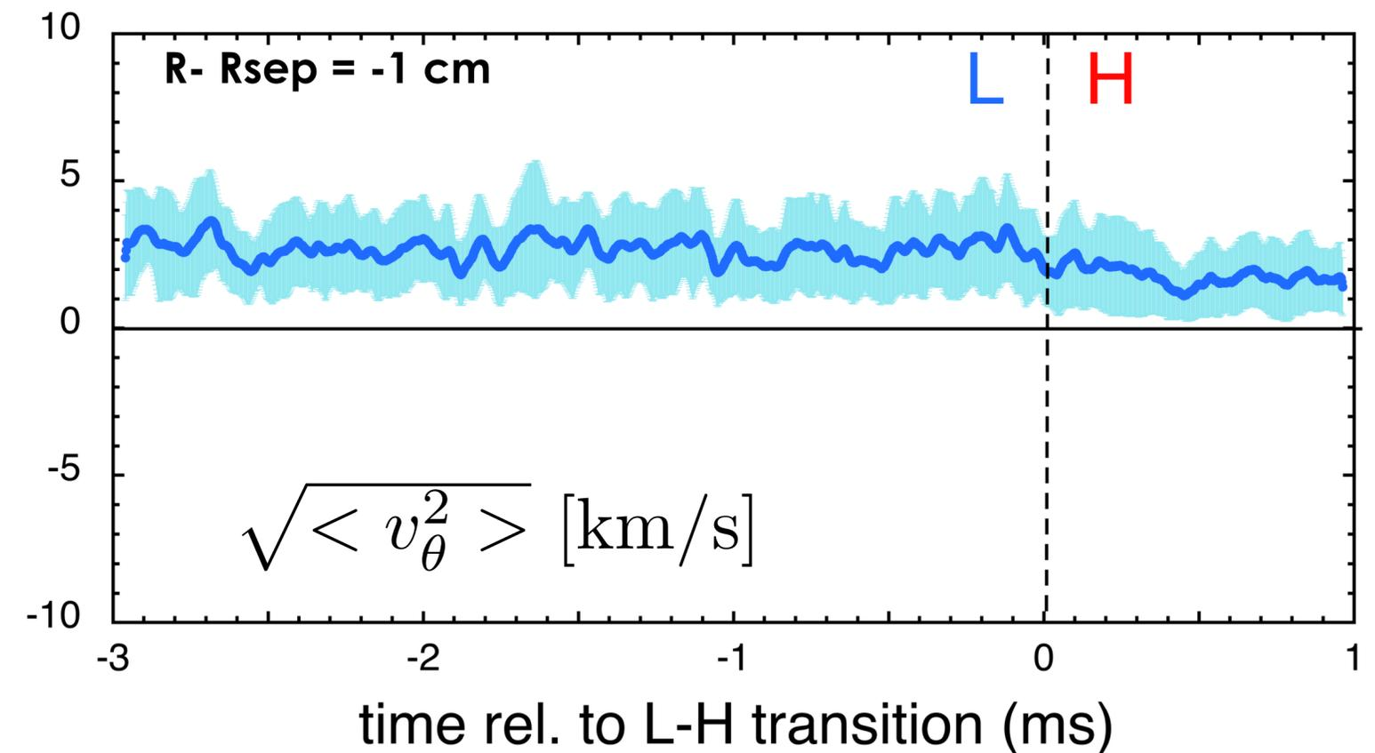
These quantities are averaged in poloidal angles and in time (over  $30 \mu\text{s}$ ) and over multiple shots
