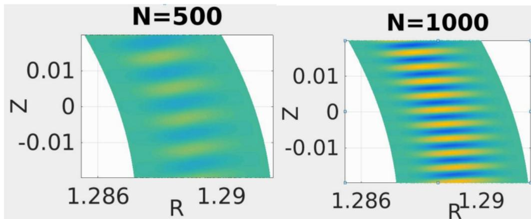
Mode structures of ETG for different  $n$ . The mode structure becomes finer as the mode number increases. Computationally very expensive.
