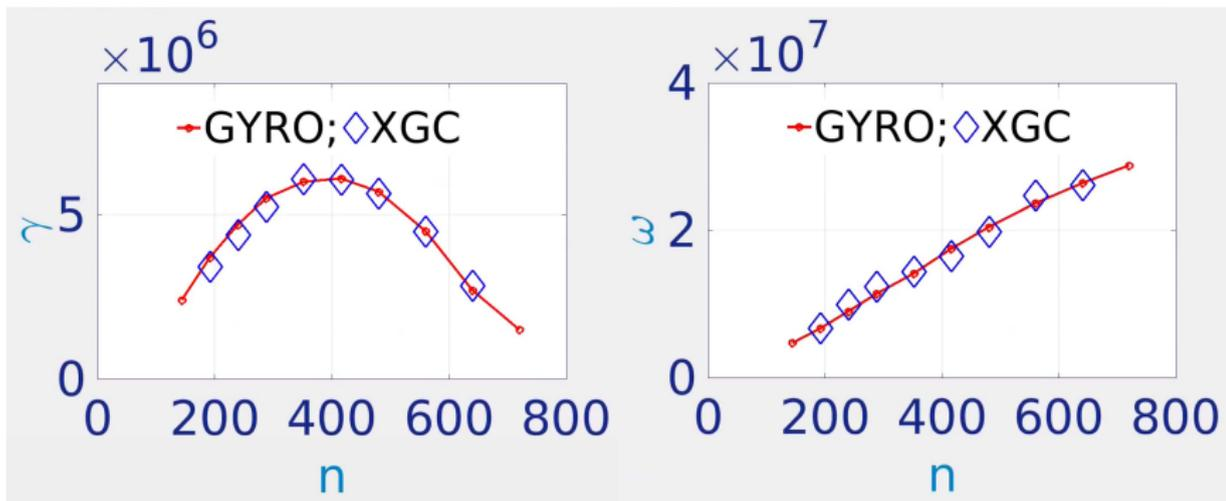
Growth rates and real frequencies for XGC1 and GYRO simulations
