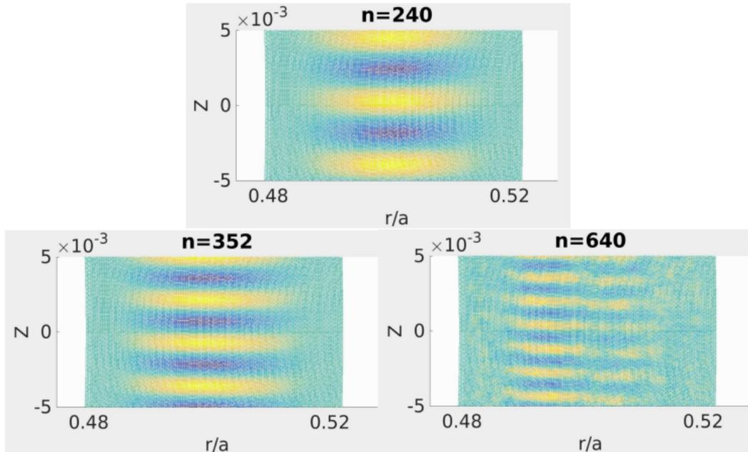
Mode structures of ETG for different  $n$ . The mode structure becomes finer as the mode number increases. Demand higher resolutions and are computationally very expensive.
