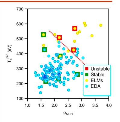
ELITE analysis showed that ELMs were consistent with peeling-ballooning triggers
