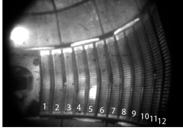
Fig 1a. View of the antenna array with the fast framing camera. Illuminating light coming from extinguishing plasma. Figs 1b and 1c have Li-I filter in place to observe excited Li neutrals.
