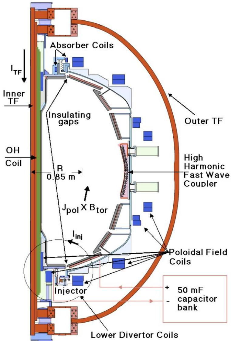
Long-pulse (400ms) CHI discharges in a 'stuffed-injector' current mode used to ablate Low-Z impurities from lower divertor
