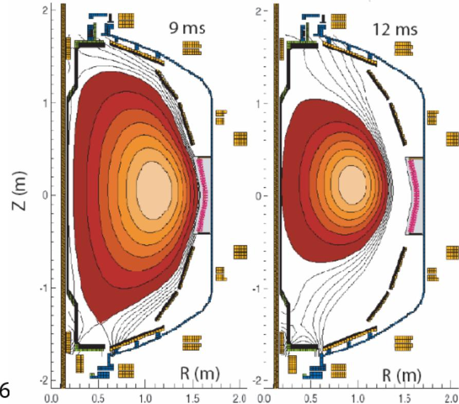
After CHI is OFF, 160kA of non-inductively generated closed flux current is present
