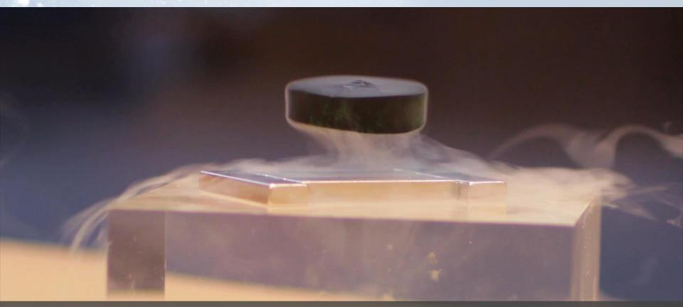
Ceramic superconductor, cooled to -196°C in liquid nitrogen, floats above very strong magnets.
