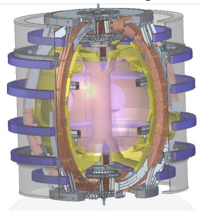
• ST40 has, like START&MAST, in-vessel merging-compression coils and only small solenoid 8
