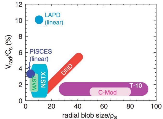
**Figure 3.** Turbulence filament cross-section size and radial velocity in the SOL normalized to the local ion Larmor radius at the electron temperature,  $\rho_s$ , and the local ion sound speed,  $c_s$ , for a number of devices.
