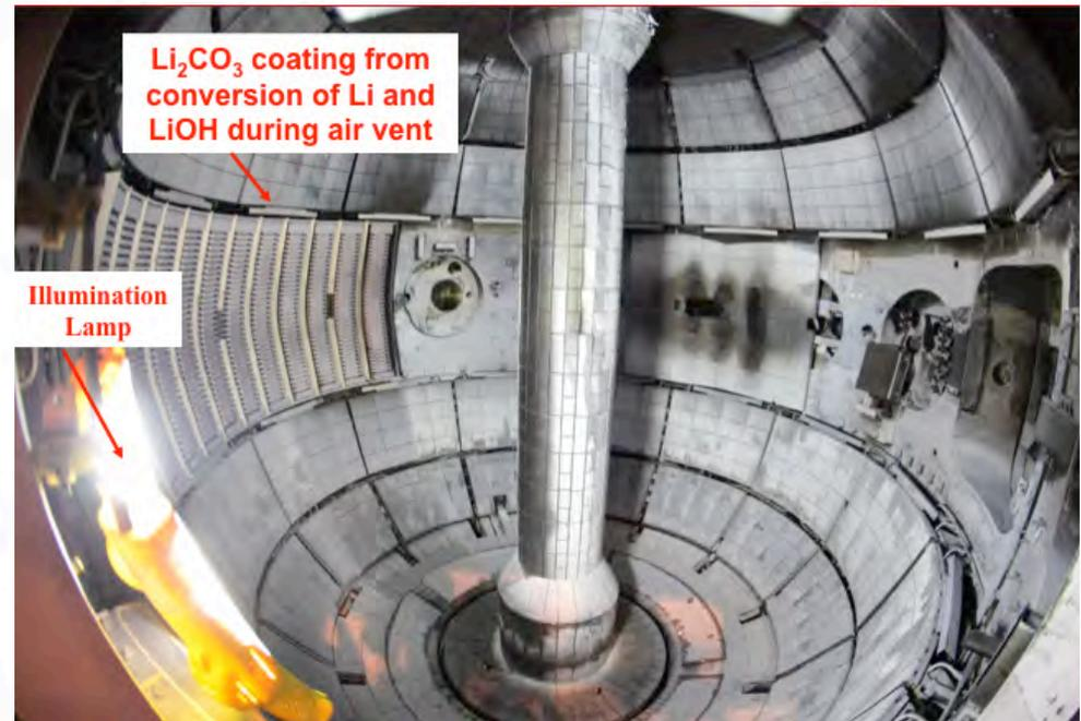
*Photo of NSTX interior following 1.3 kg lithium deposition applied during 2010-2011 experimental campaigns indicating extensive lithium coverage due to direct evaporation and plasma transport*
