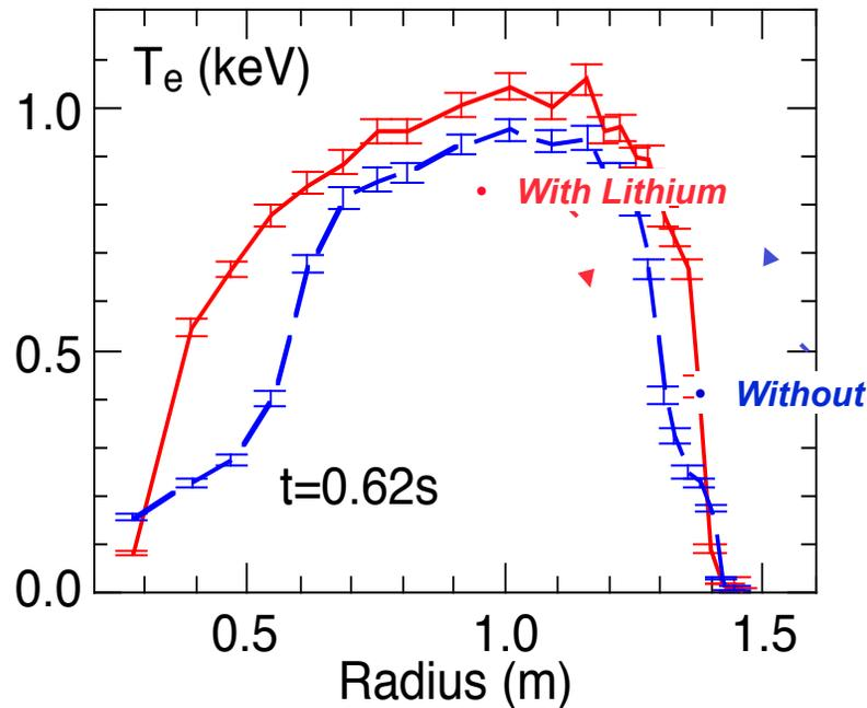
Radial profiles of electron temperature before (blue) and after 260 mg lithium deposition (red) in the NSTX H-mode discharges.
