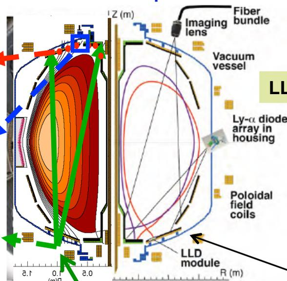
**Two fast 2D visible and IR cameras with full divertor coverage**
