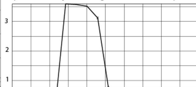
Representative Injector Current Waveform (Arbitrary Units)
