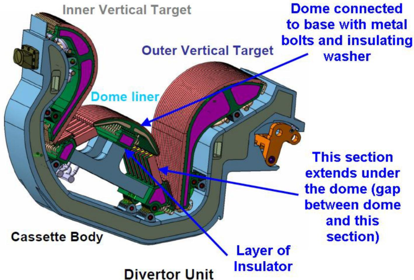
**Insulator is under compression and shielded from neutron**
