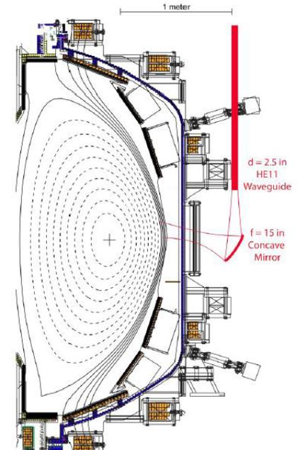
28 GHz ECH/EBWH waveguide
