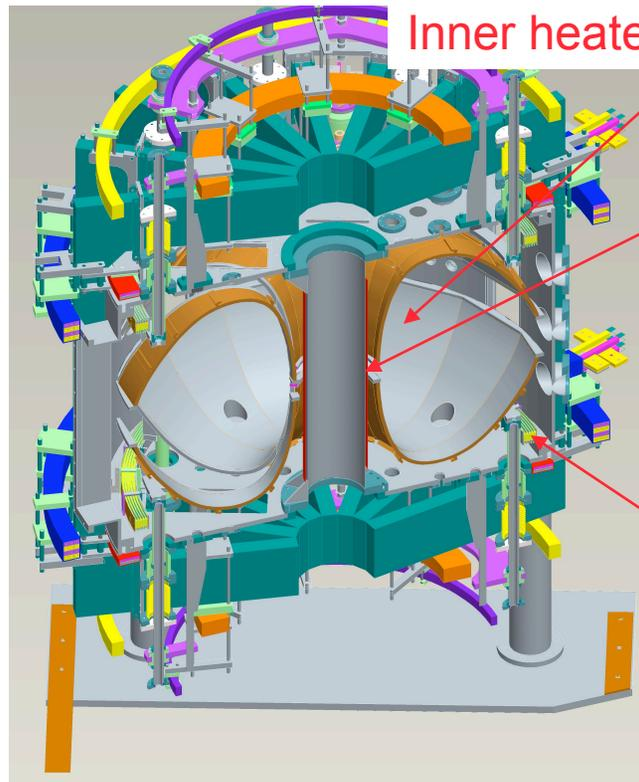
Inner heated shell (explosively bonded SS on copper)
