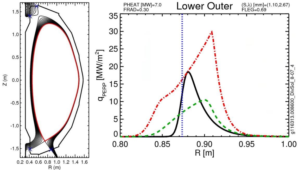
**Figure 2:** Equilibrium which drives OBD-R3 requirement for CASE#1 and the heat flux profile modeling (right). The green-dashed line is the time-averaged heat flux, assuming fast sweeping, while the red is the peak encountered over the scan
