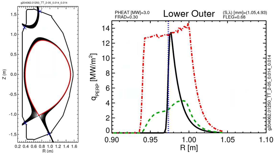
Figure 1: Equilibrium which drives OBD-R4 requirement for CASE#1 and the heat flux profile modeling (right). The green-dashed line is the time-averaged heat flux, assuming fast sweeping, while the red is the peak encountered over the scan.
