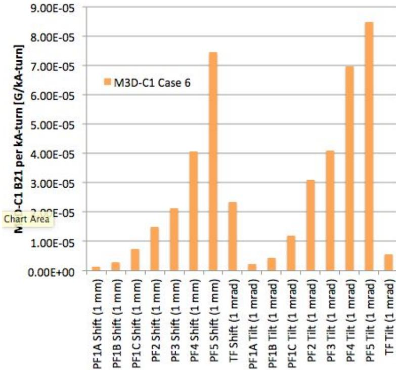
Figure 3.2.2-4: Dependence of  $B_{21}$ , for full coil kA-turns on the TF and PF coils and 100 A on the RWM coils, on individual coil tilts and shifts in two L-mode cases using M3D-C1.
