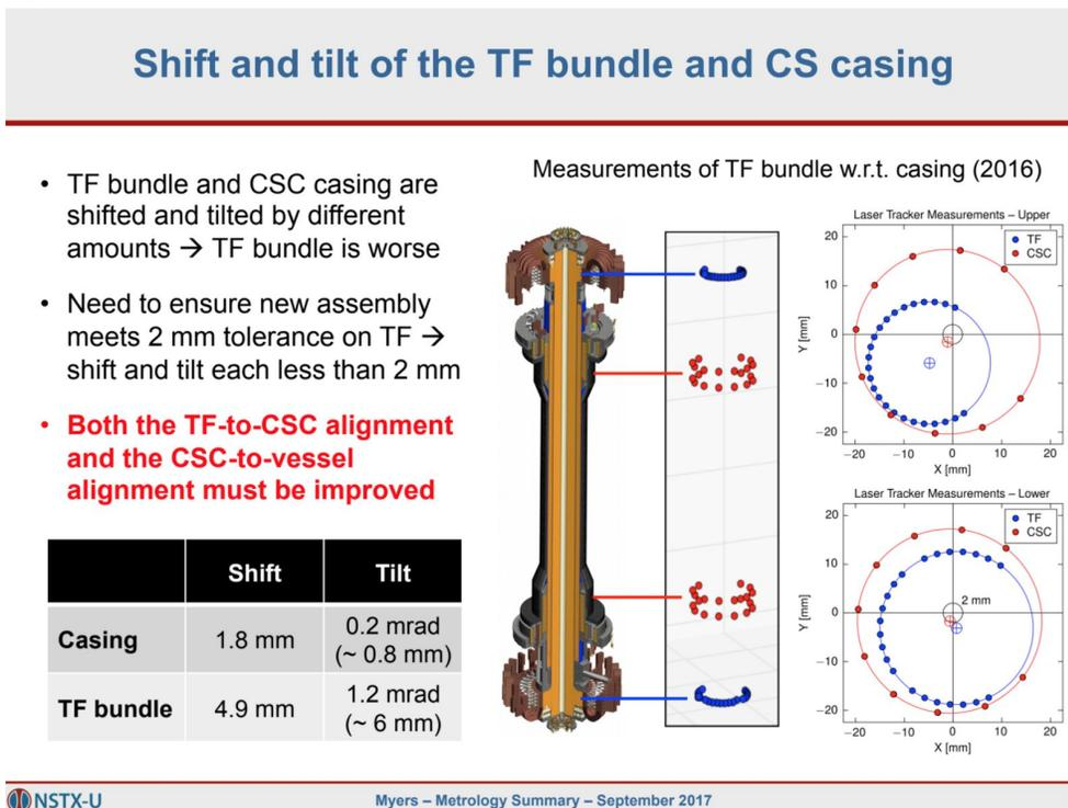
It was found that the bundle had a significant (1.2 mrad) tilt within the casing. It should be noted that no effort was made during installation to fix this tilt, and the presence of the tilt in that assembly does not imply that it could not have been corrected.
