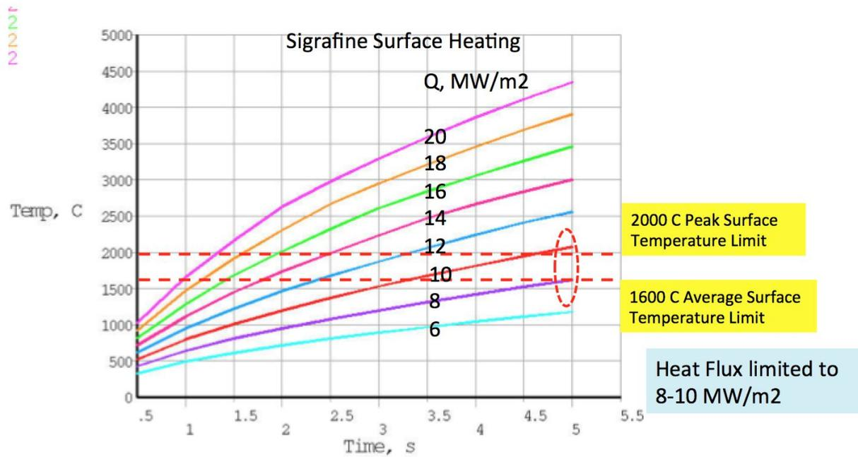
**Figure 2.0-1:** Surface temperature as a function of time, for various heat flux values, under a 1D assumption. This figure is from Ref. 6, and uses the thermal conductivity of a specific material.
