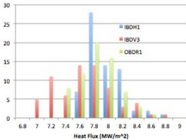
**Fig. 2.2.6-1:** Histogram of Monte-Carlo results for the case in Table 2.2.6-1.
