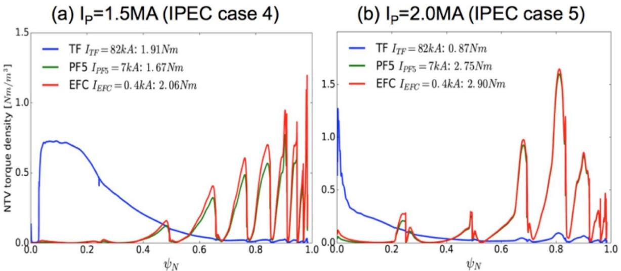
It should be noted, however, that NTV is a profile effect, with the values in Fig. 3.2.1-1 and 3.2.1-2 being integrated over the plasma volume to provide the total torque. Examples profiles are shown in Fig. 3.2.1-3, for the TF displacements and PF-5 radial variations observed during the FY-16 run (the measured PF-5U tilt is not included in this calculation). The NTV the RWM coils is also shown, with a magnitude selected to match that from the PF-5 perturbation. It is
