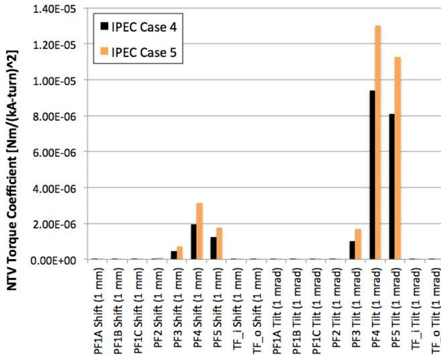
**Figure 3.2.1-2:** Dependence of  $T_{NTV}$  for full coil kA-turns on the TF and PF coils and 100 A on the RWM coils, on individual coil tilts and shifts using IPEC. The equilibrium is the Case 4 H-mode case.
