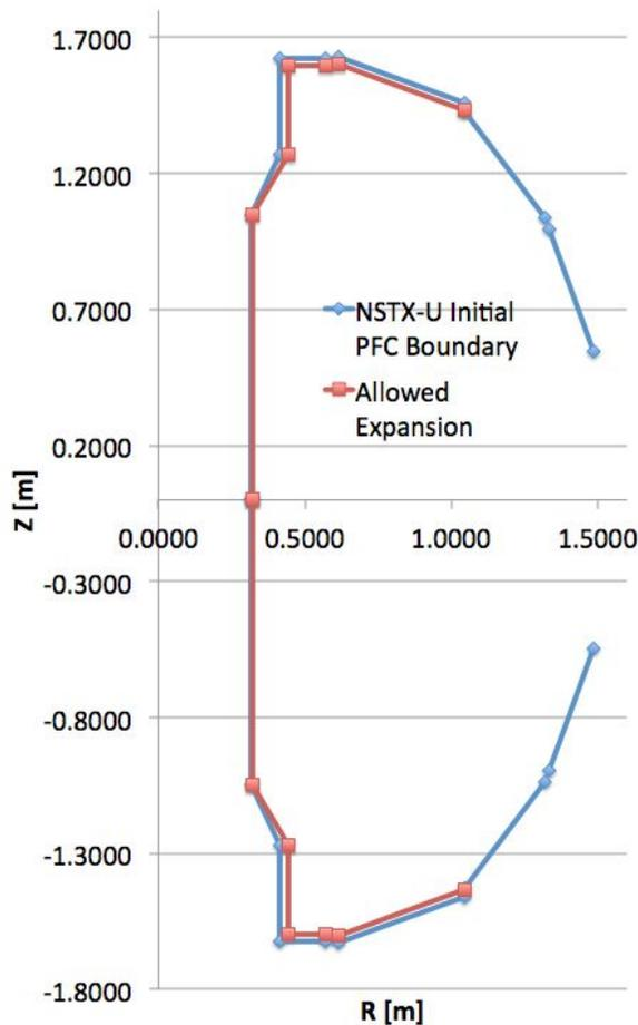
**Figure 2.5.1:** NSTX-U PFC boundary and allowed expansion of PFCs to accommodate new requirements
