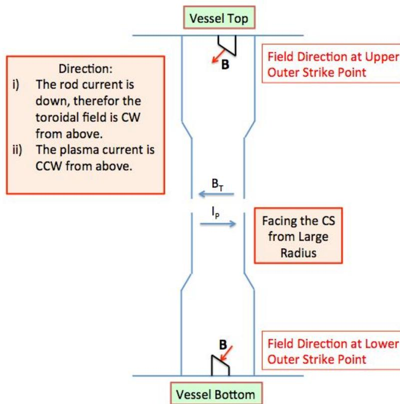
**Fig: 3.2.1:** Field line direction on the horizontal target for “Standard Helicity”
