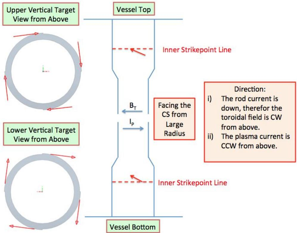
Fig: 3.3.1: Field line direction on the vertical target for "Standard Helicity"
