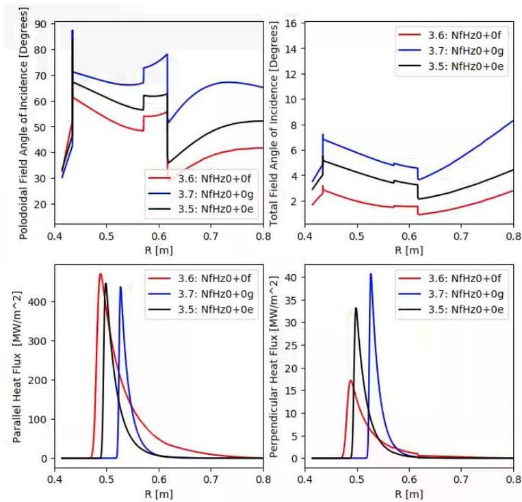
**Fig. 3.2.4:** Heat flux profiles for standard divertors placing heat on the inner target. Sweeping is allowed for these cases to qualify 5 second operations.
