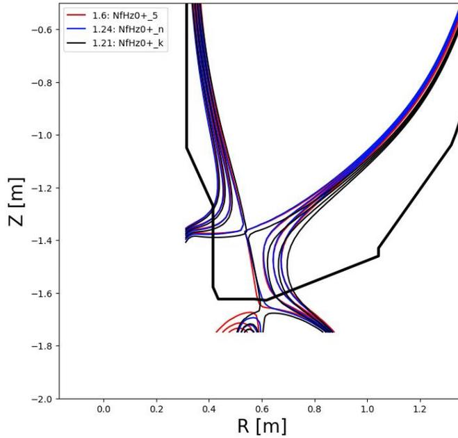
**Fig. 3.4.1:** Stationary high flux expansion divertor geometry placing heat on the outer target.
