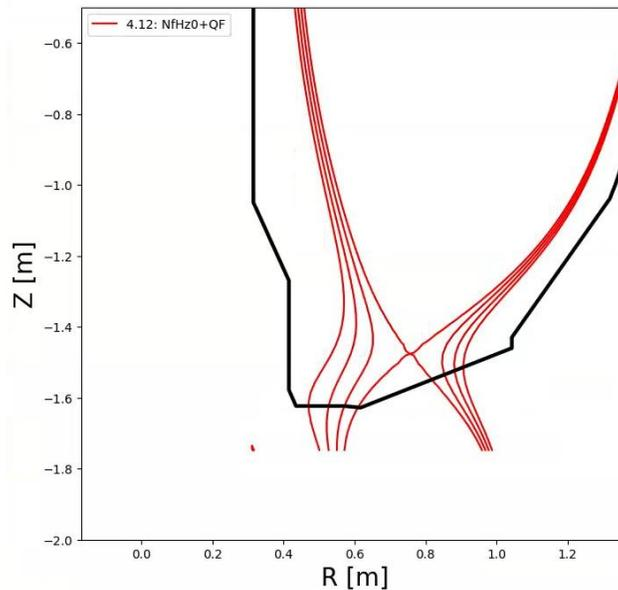
**Fig. 3.2.5:** Low triangularity equilibrium. This case has reversed target helicity on the inboard horizontal target.
