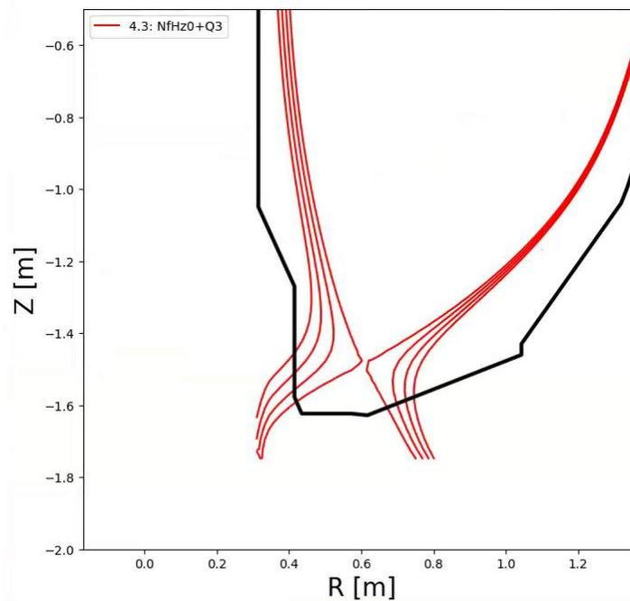
**Fig. 3.4.3:** Low-triangularity equilibrium placing heat on horizontal inner target (Section 3.2.3) and the middle of the outer target.
