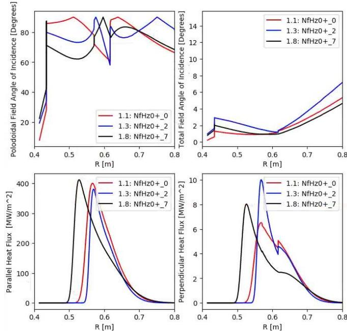
**Fig. 3.2.2:** Stationary divertor profiles for high flux expansion scenarios placing heat on the inner target.
