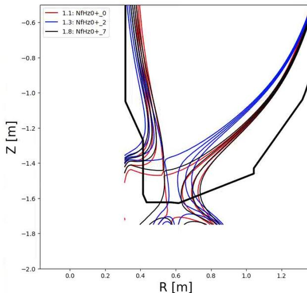
**Fig. 3.2.1:** Stationary high flux expansion divertor geometry placing heat on the inner target.
