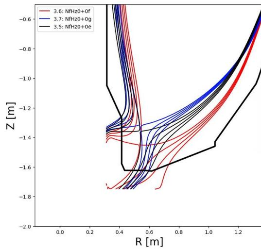
**Fig. 3.2.3:** Standard divertor geometry placing heat on the inner target. Sweeping is allowed for these cases.
