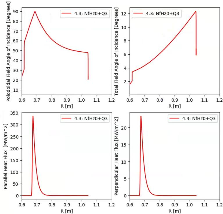
**Fig. 3.4.4:** Heat flux profiles for low-triangularity equilibrium placing heat on horizontal inner target (Section 3.2.3) and the middle of the outer target.
