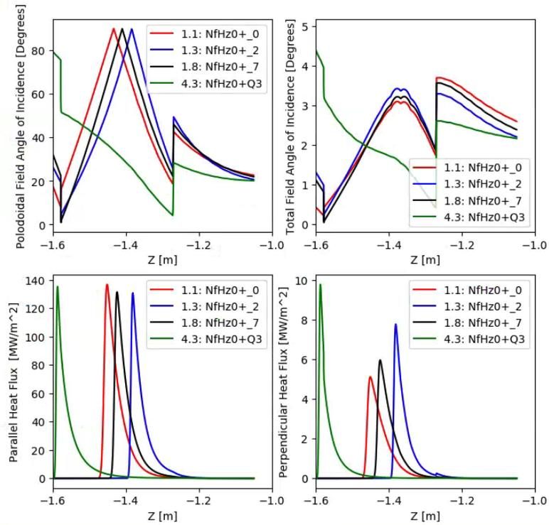
**Fig. 3.3.2:** Heat flux profiles on the vertical target.
