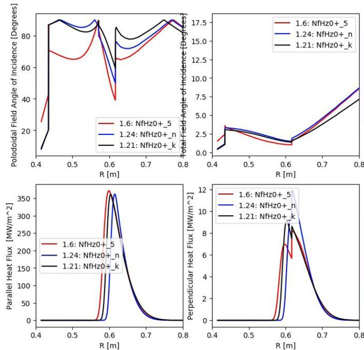
**Fig. 3.4.2:** Stationary high flux expansion divertor geometry placing heat on the outer target.
