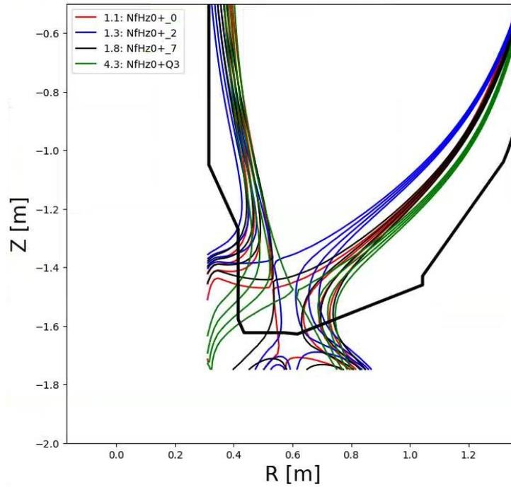
**Fig. 3.3.1:** Heat flux profiles on the vertical target.
