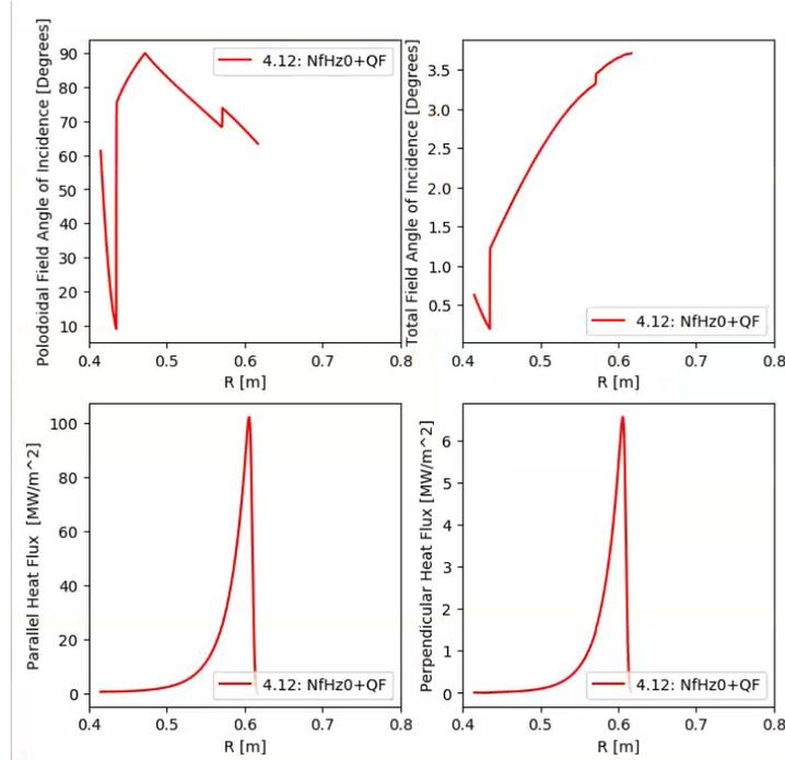
**Fig. 3.2.6:** Inboard horizontal target profiles for case with ISP on the horizontal target. This case has reversed target helicity on the inner horizontal target. Note that a DN power split on the inner leg is assumed, unlike in the excel spreadsheet.
