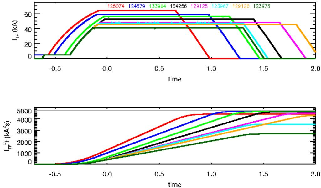
Figure #2: Example TF waveforms, along with their approach to the  $I^2t$  limit of the coil.
