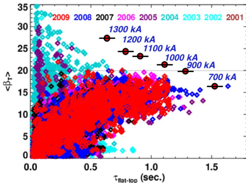
Fig 1: The NSTX database of flat-top average  $\beta_T$  values, sorted by year. Also shown in red circles are the target points for this XP at  $B_T=0.4T$ , assuming good confinement.
