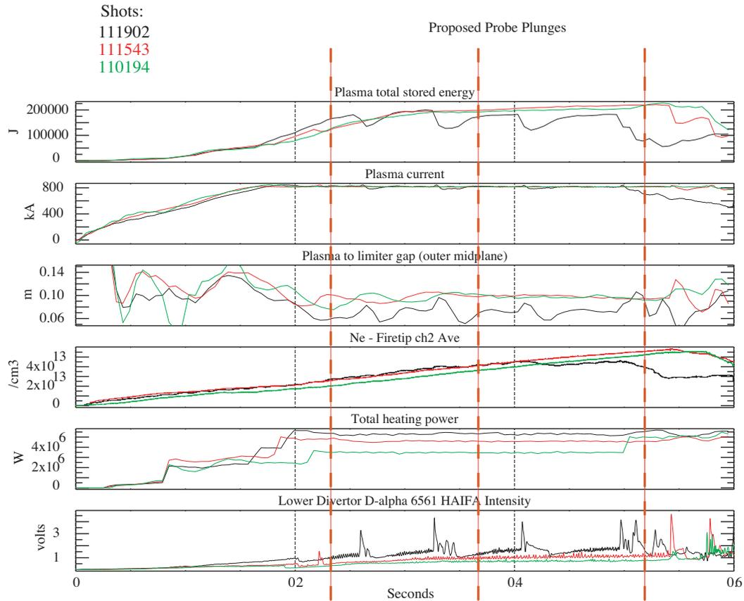
Figure 4. Timeline for reference shots 110194, 111543 and 111902. Proposed discharges have lower power levels. H-mode transition will be avoided by LFS gas puff. The probe will plunge at various times during the discharge to sample different densities.
