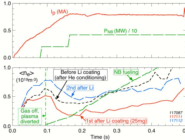
Lower single-null divertor discharges, 0.45T, D<sub>2</sub> gas fueled 3.5mg
