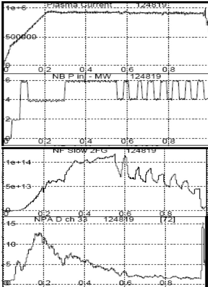
Shot 124819 is from XP 737. However, the NPA channels show no correlation with the beam modulations and neutron signals, even at the highest channel. This may be due to the NPA sightline viewing outside of the beam deposition region. The expectation is that if the NPA sightline is adjusted, the modulations will be visible.
