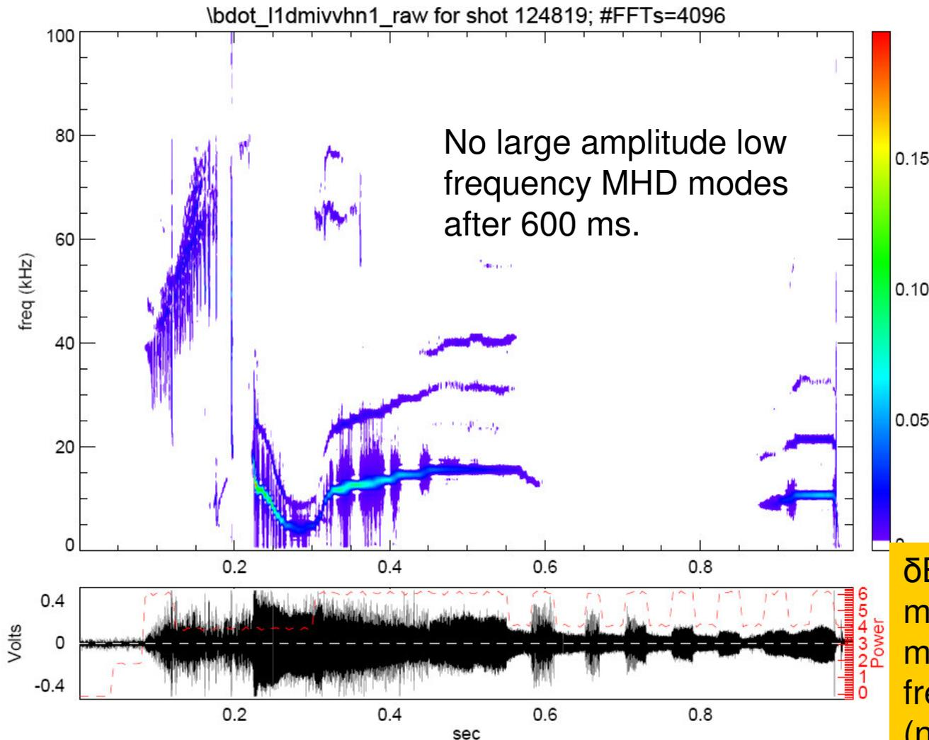
This shot is useful because it has a reproducible MHD free period, which is critical in determining the fast ion distribution.
