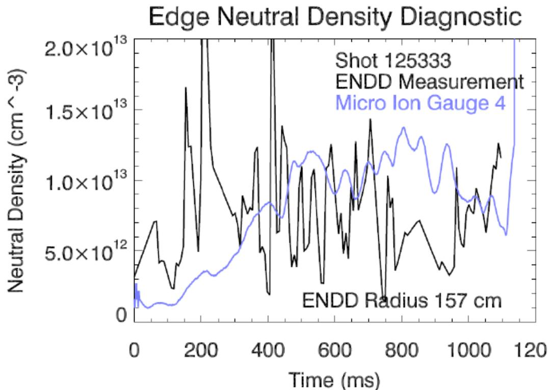
The Edge Neutral Density Diagnostic is working and was compared with a micro ion gauge to verify results.
