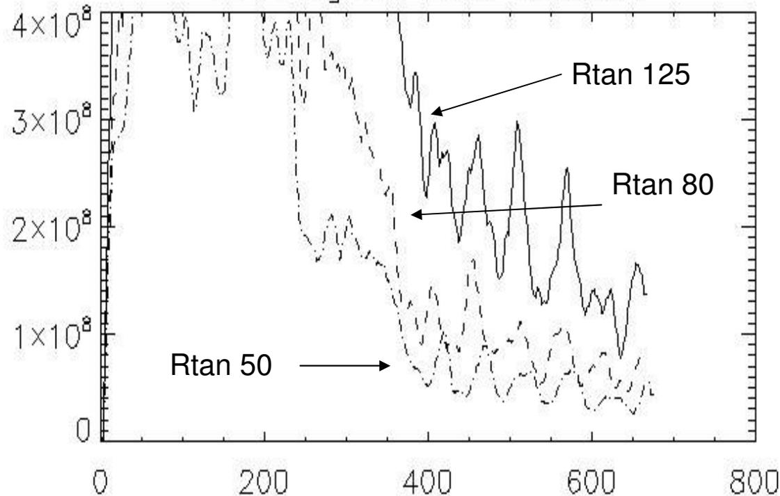
TRANSP shows modulations at all tangency radii that match the beam modulations. This is not seen in the measured NPA signal, particularly for Rtan 80, near the magnetic axis. (The measured NPA signal is not shown)
