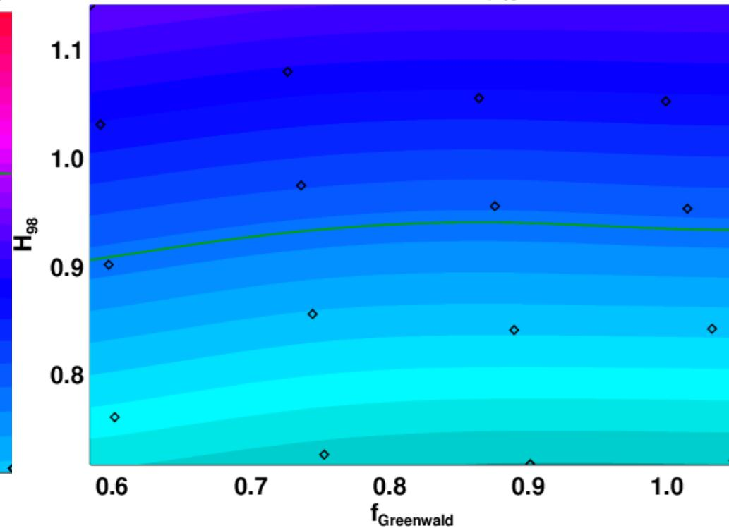
1.0 T, 900kA,  $A=1.65$ ,  $\kappa=2.7$ ,  $R_{\text{tan}}=[50,60,70,110,120,130]$  90 kV Beams
